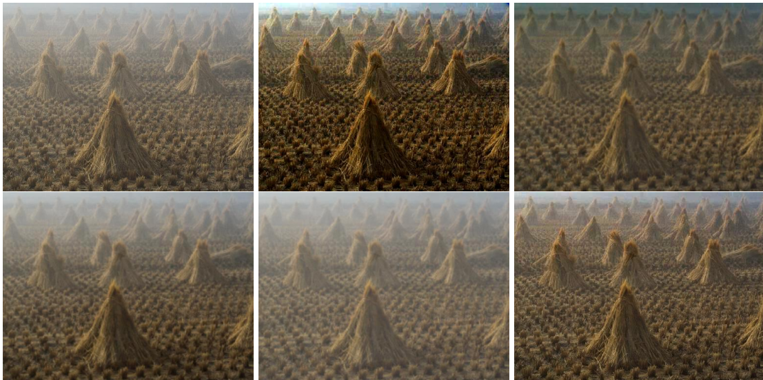
Figure 6.5: Top left is the original image, top middle image dehazed using VarDCP, and top right using Unsupervised DCP. Bottom left is dehazed using FFANet, bottom middle using Dehazeformer, and bottom right using MSCNN. Note that the biggest improvements seem to be from the VarDCP method and the unsupervised DCP method, while the smallest improvements seem to come from the FFANet and Dehazeformer.
