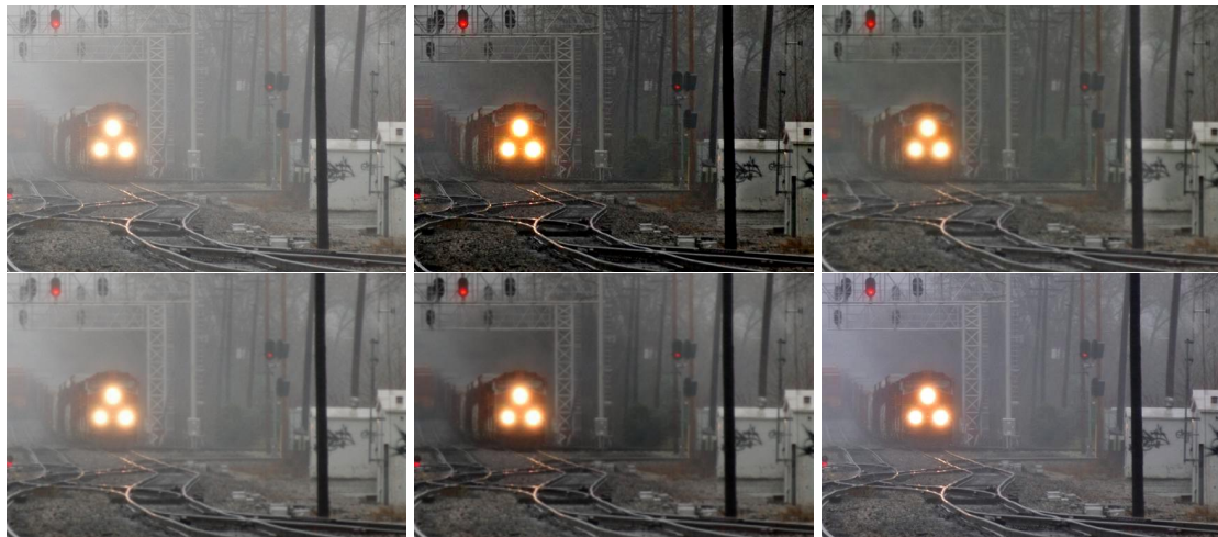
Figure 6.7: Top left is the original image, top middle image dehazed using VarDCP, and top right using Unsupervised DCP. Bottom left is dehazed using FFANet, bottom middle using Dehazeformer, and bottom right using MSCNN. The biggest improvement here comes from the Dehazeformer, followed by the VarDCP method. This image is particularly interesting because the headlights of the train do not conform to the haze degradation model well.
