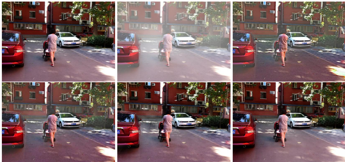
Figure 6.2: Example of an image from the outdoor portion of the testing set. In the top row are the ground truth on the left, then the generated hazy image, and then the image dehazed using the Unsupervised DCP method. In the bottom row are images dehazed using the Variational DCP method on the left, FFANet in the middle, and Dehazeformer on the right. Here, the supervised methods heavily outperform the proposed methods.
