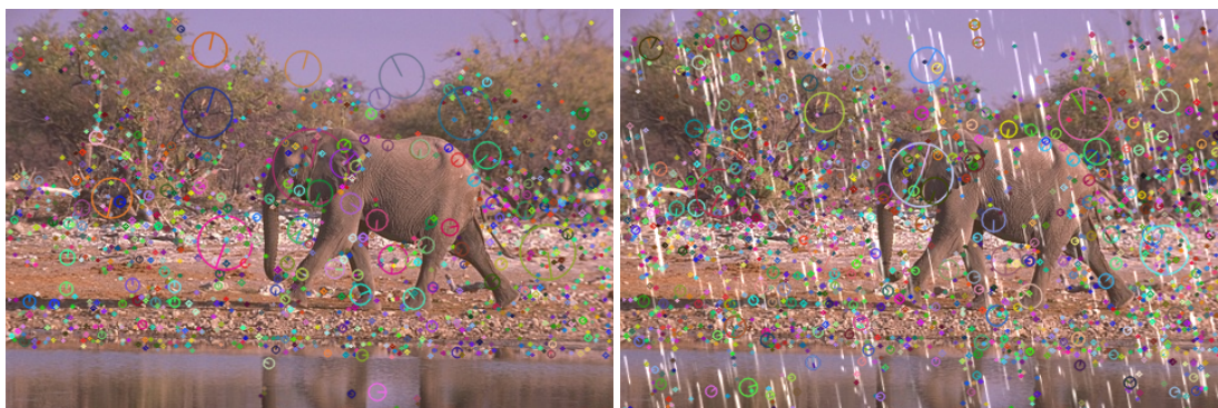
Figure 1.1: SIFT features calculated on an image without rain (left) and on an image with rain (right). Note how many of the detected features are actually features of rain rather than the scene itself.
