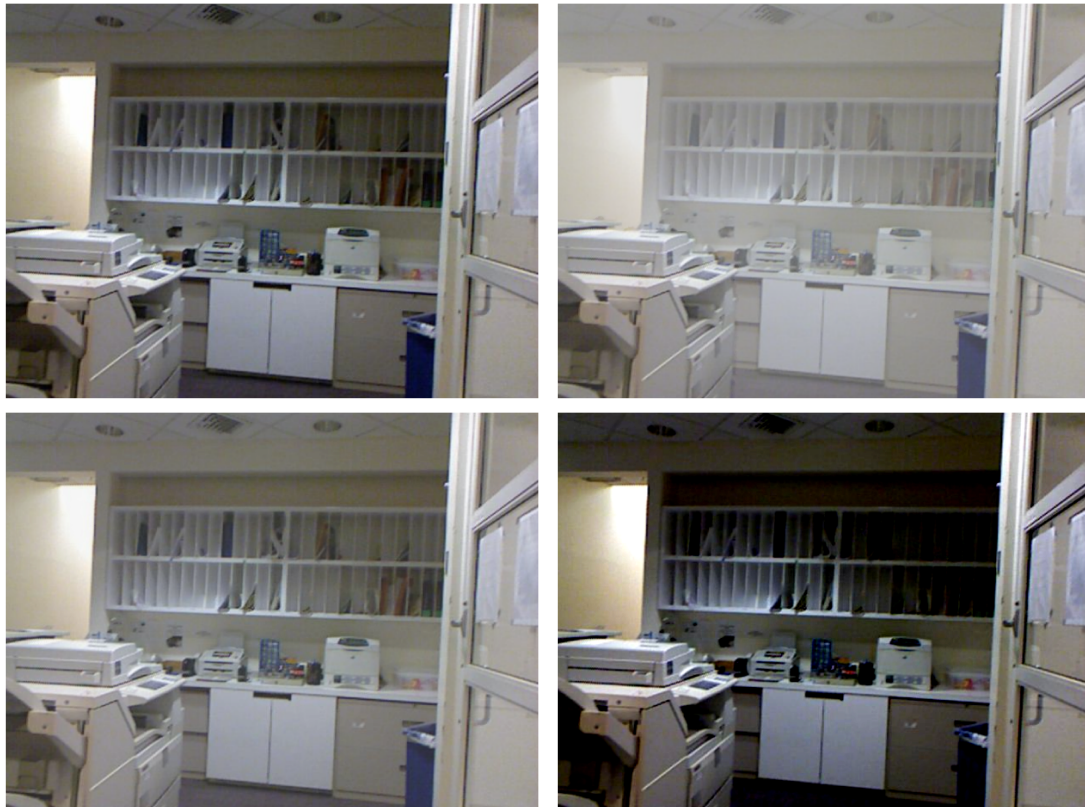
Figure 4.1: An example of the effects of overestimating and underestimating the transmission map t . The top left is the original clear image with known depth for each pixel. The top right is a hazy image made using equation (1.20) and depth information of the image. The bottom left is the image reconstructed by underestimating t by 25% at every pixel, while the bottom right is made by overestimating by the same amount.
