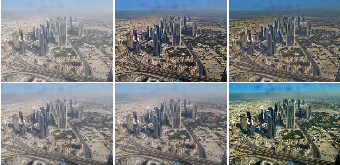
Figure 6.9: Top left is the original image, top middle image dehazed using VarDCP, and top right using Unsupervised DCP. Bottom left is dehazed using FFANet, bottom middle using Dehazeformer, and bottom right using MSCNN. FFANet and Dehazeformer once again do not change the image. The best results come from VarDCP and the Unsupervised DCP.
