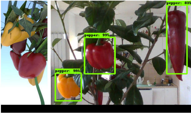
Fig. 4 a) Example of a synthetic pepper image generated in Blender software. b) Example of detected sweet peppers in an Intel RealSense 2D image, with the bounding boxes used in point cloud filtering. The image shows one real example for all of the pepper varieties used in this work: a yellow bell pepper on the left, a red bell pepper in the middle, and a red horn variety pepper on the right
