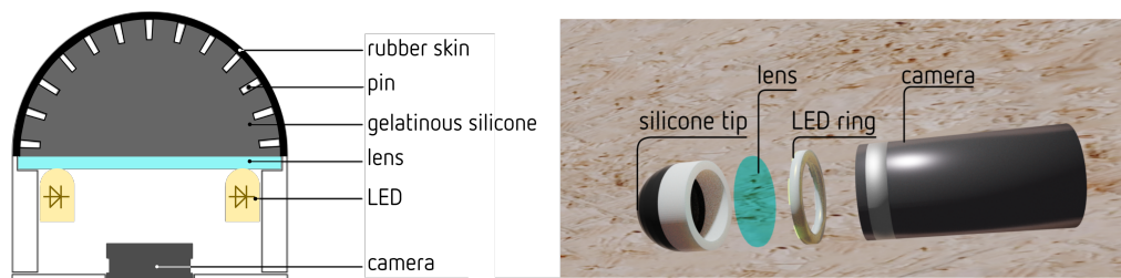
Figure 2.2: Cross-section and 3D schematic of the basic TacTip architecture.
