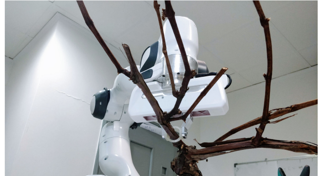
Fig. 1. Collaborative robot Franka Panda performing the exploration procedure on a Vitis vinifera plant stem using a rigid end-effector gripper.
