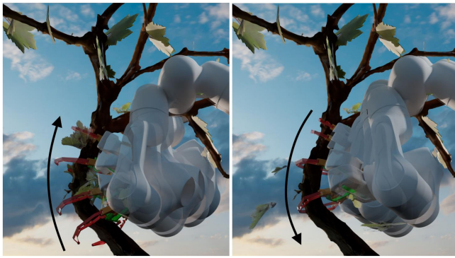
Fig. 2. Cleaning vine stems from scrubs and old rind starts with localizing and perching the plant preceding to plant exploration moving upwards. Once we reach a certain threshold, the exploration stops, the grip is tightened and the cleaning procedure starts from the top.
