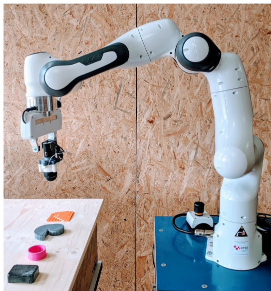
Fig. 1. Experimental setup used in dataset acquisition. The TacTip sensor is mounted on a Franka Emika 7DoF arm, and contact is realized with rigid objects of various shapes and sizes. Optoforce sensor was used to obtain force measurement dataset.
