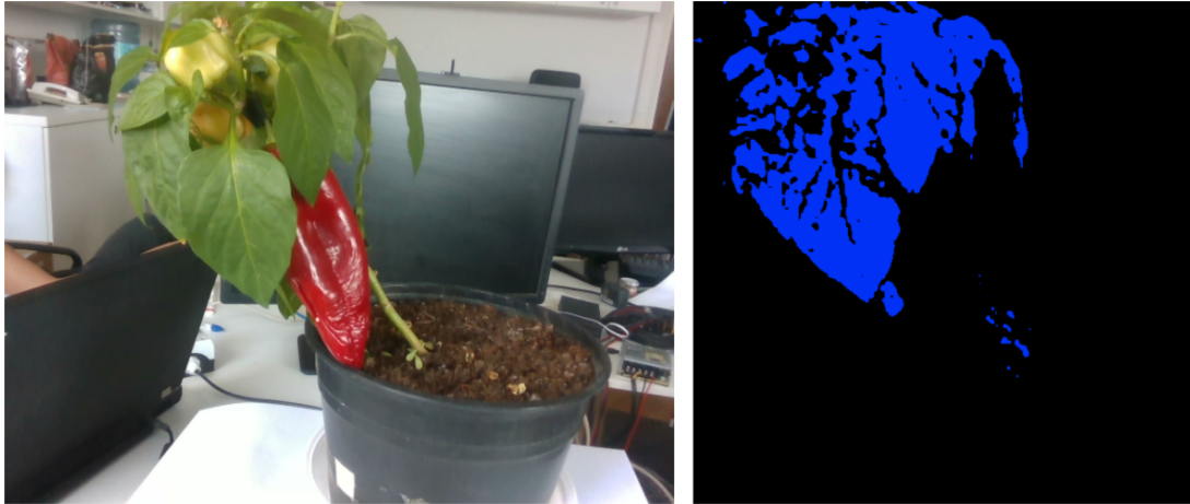
Figure 3.9: RealSense D435 RGB image of a scene with a pepper plant, and a corresponding DeepLabV3+ output semantic mask of the leaf pixels.
