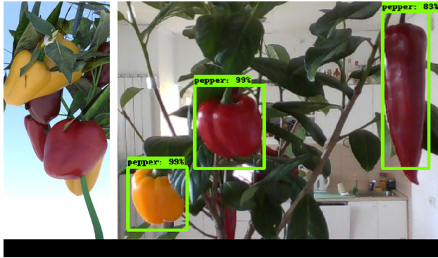
Fig. 4 a ) Example of a synthetic pepper image generated in Blender software. b ) Example of detected sweet peppers in an Intel RealSense 2D image, with the bounding boxes used in point cloud filtering. The image shows one real example for all of the pepper varieties used in this work: a yellow bell pepper on the left, a red bell pepper in the middle, and a red horn variety pepper on the right
