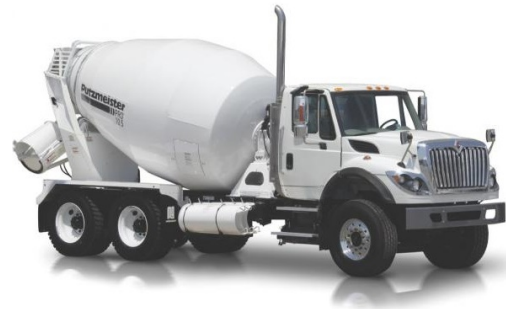
Fig. 6: Example concrete mixer truck [11]
