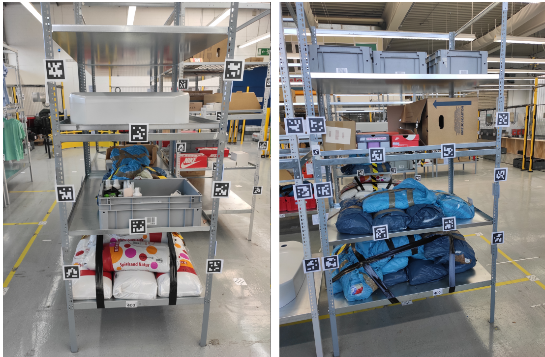
Figure 2.11: AprilTags placed throughout the testing arena for acquiring the ground truth pose information. All AprilTags are unique and their map is computed with TagSLAM package.
