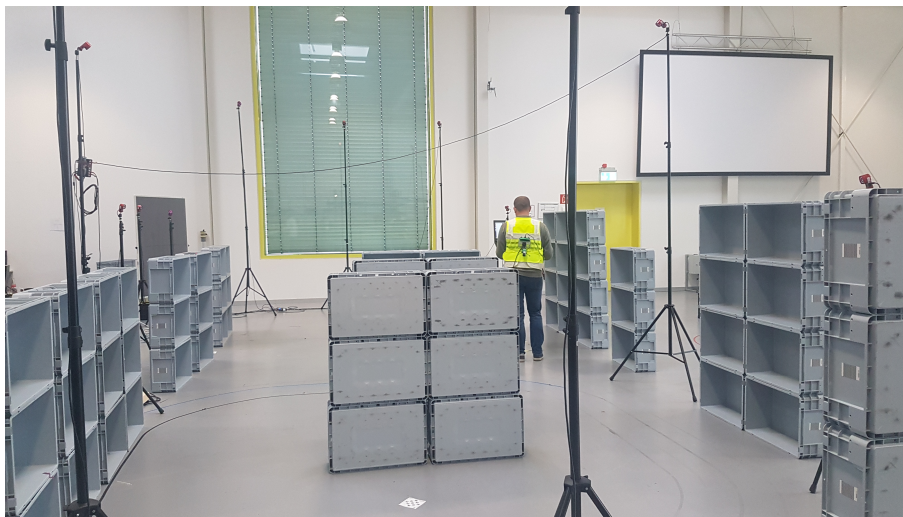
Figure 2.9: The experimental arena for collecting Dortmund dataset. The plastic boxes imitate racks and walls. The arena is covered with Optitrack motion capture system. (By courtesy of Fraunhofer IML).
