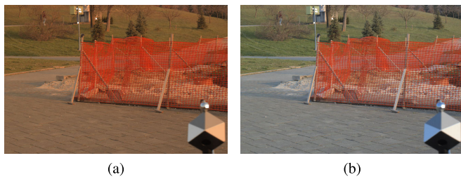
FIGURE 12. Example of chromatic adaptation based on illumination extracted from a) left and b) right gray face of the SpyderCube calibration object placed in the scene.
