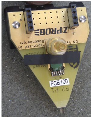
(a) Initial wafer probe design.
