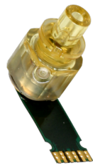
(a) TOSA package with the flexible PCB.
