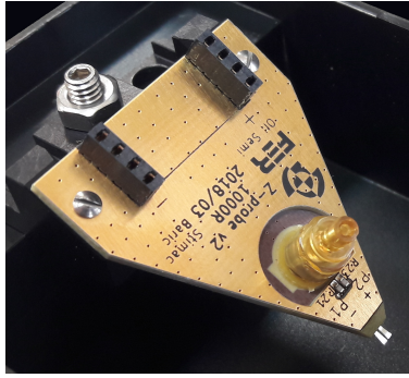
(a) Floating-ground probe design (top).
