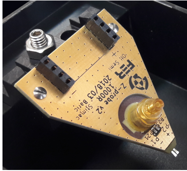
(a) Floating-ground probe design (top).
