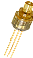
(b) Through-hole TOSA package.
