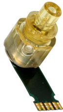
(a) TOSA package with the flexible PCB.
