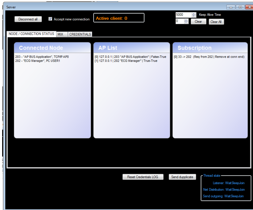
Figure 4-2 Central server application with a list of connected nodes, access points list and subscription list.
