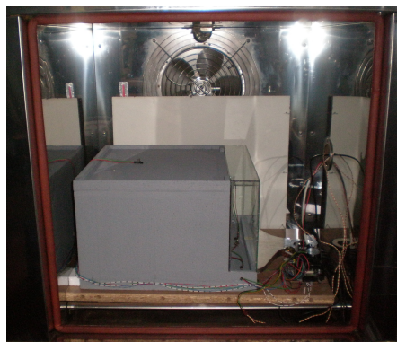
FIGURE 2.29. Thermal chamber with the scaled mock-up inside the chamber
