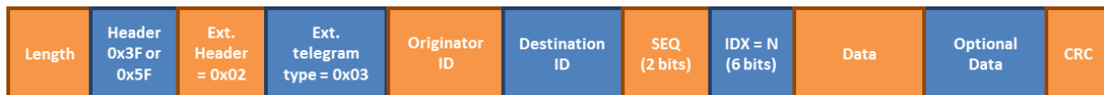
Figure 3.39. The content of the second and each further split parts of the chained telegram.
