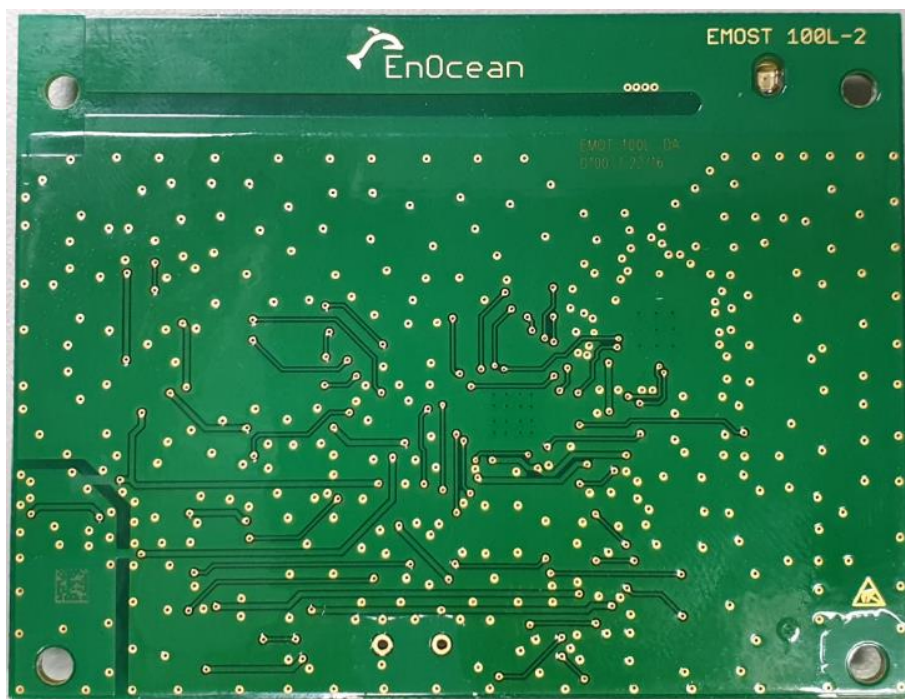
Figure 2.64. Assembled data logger module PCB (bottom view).
