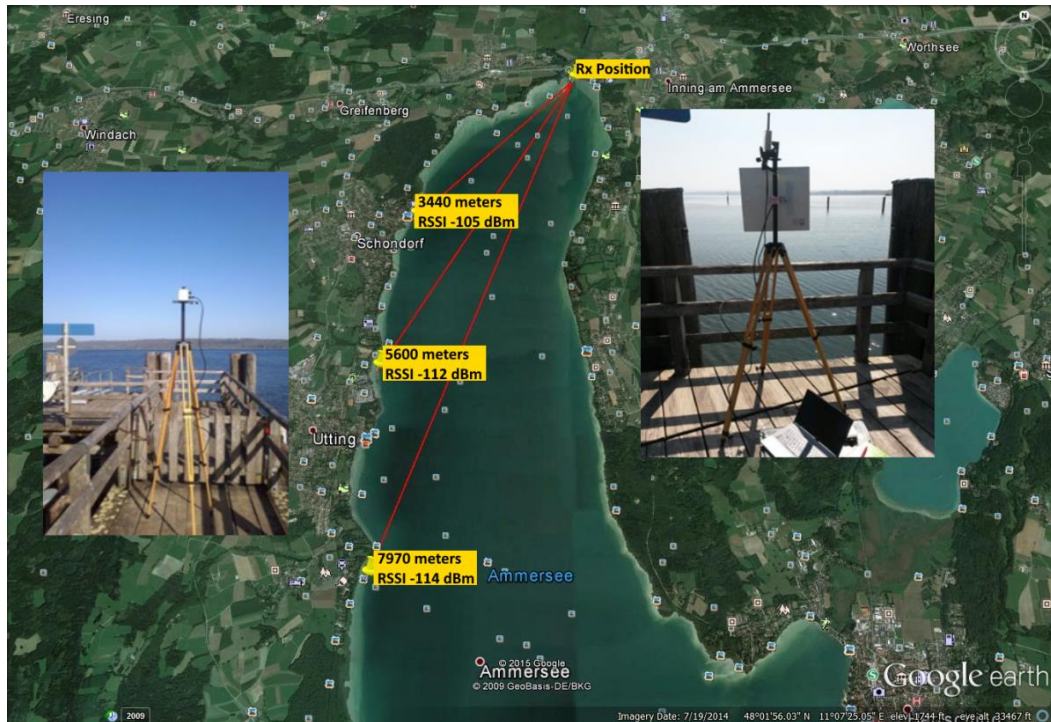
Figure 5.6. Range tests at lake Ammersee (south Germany) with the ~ 8 km achieved transmission range. The data logger module was equipped with the high gain antenna shown on the right (+12.5 dBi) and the sensor module (shown on left) with the integrated PCB antenna (~ 0 dBi).
