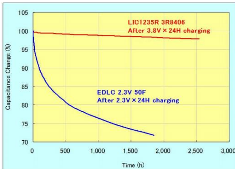
Figure 2.20. Self-discharge property of the cylinder type LIC with 40 F vs. EDLC with a similar capacitance [32].
