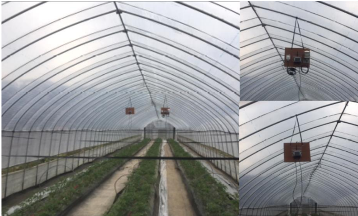
Figure 5.23. Sensor modules installed in a greenhouse to monitor conditions during tomato growth. The sensor module hanging on the left (zoomed down) has soil moisture and soil temperature sensors attached, while the sensor module on the right (zoomed up) has illuminance and air temperature and humidity sensor attached.
