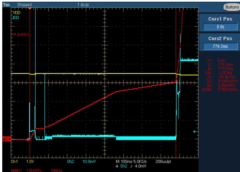
Figure 4.8. Operations executed before the 1 st data subtelegram transmission and the energy consumed during this time. The total time between the two red markers is 779.2 ms and the energy consumed during this time is 3 mWs. After the second red marker, the red curve starts to quickly ascend, representing the beginning of the 1 st subtelegram transmission.
