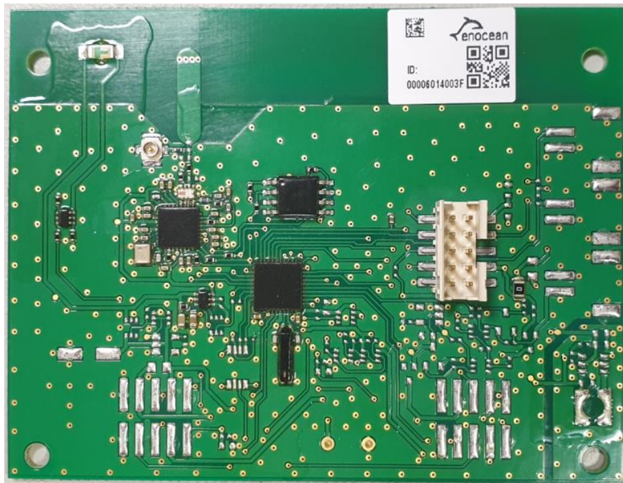
Figure 2.63. Assembled data logger module PCB (top view).
