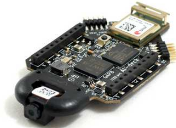
Figure 5.3: AI Deck - camera used in performing inspection
