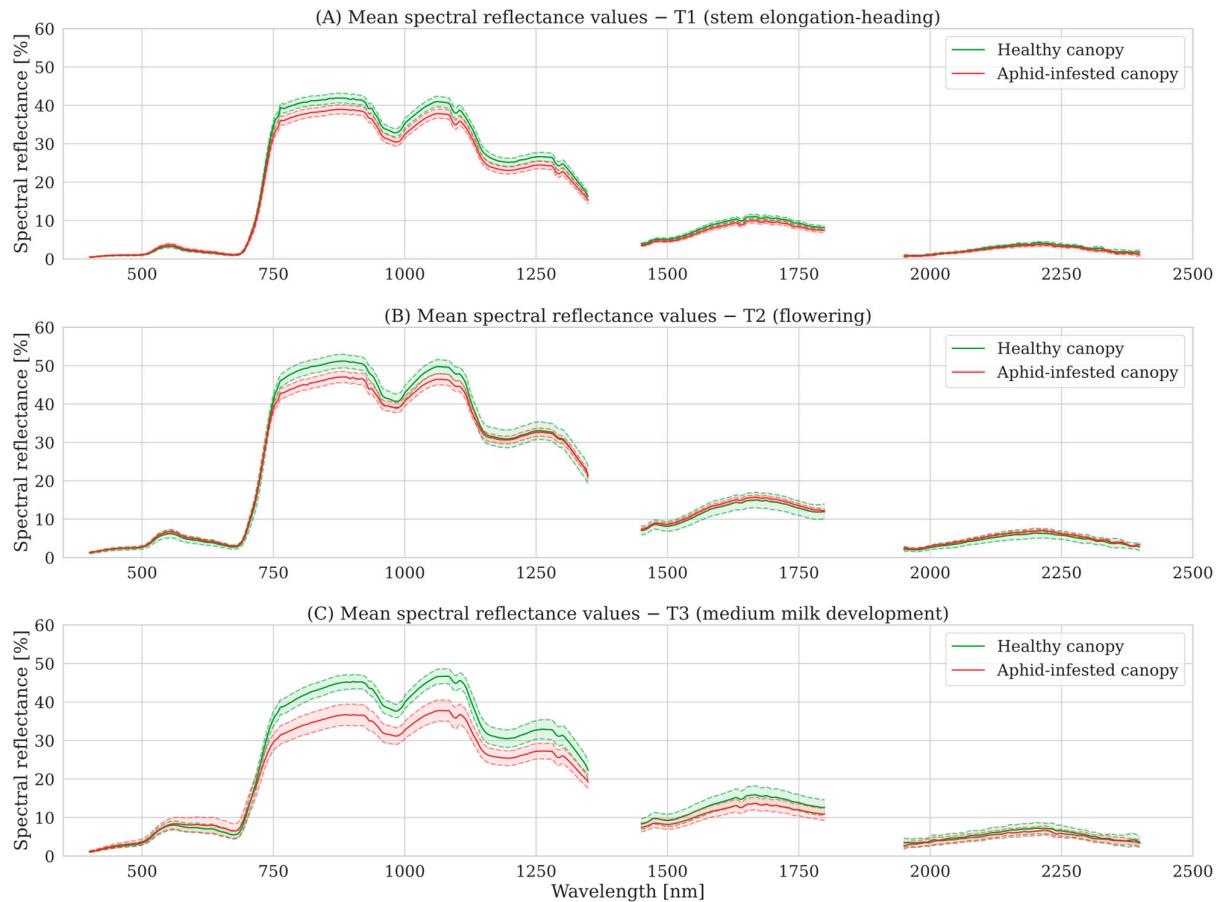
Figure 3. Mean and standard deviation of canopy spectral reflectance curves for healthy (green) and aphid-infested (red) winter wheat canopies across three growth stages: (A) T1—stem elongation-heading (BBCH 30–55), (B) T2—flowering (BBCH 55–59), and (C) T3—milky grain development (BBCH 69–75). Each mean spectral reflectance curve is based on 145 samples for T1, 141 samples for T2, and 145 samples for T3. Spectral regions affected by atmospheric noise (1350–1450 nm, 1800–1950 nm, and 2400–2500 nm) and non-informative content (350–400 nm) were excluded.
