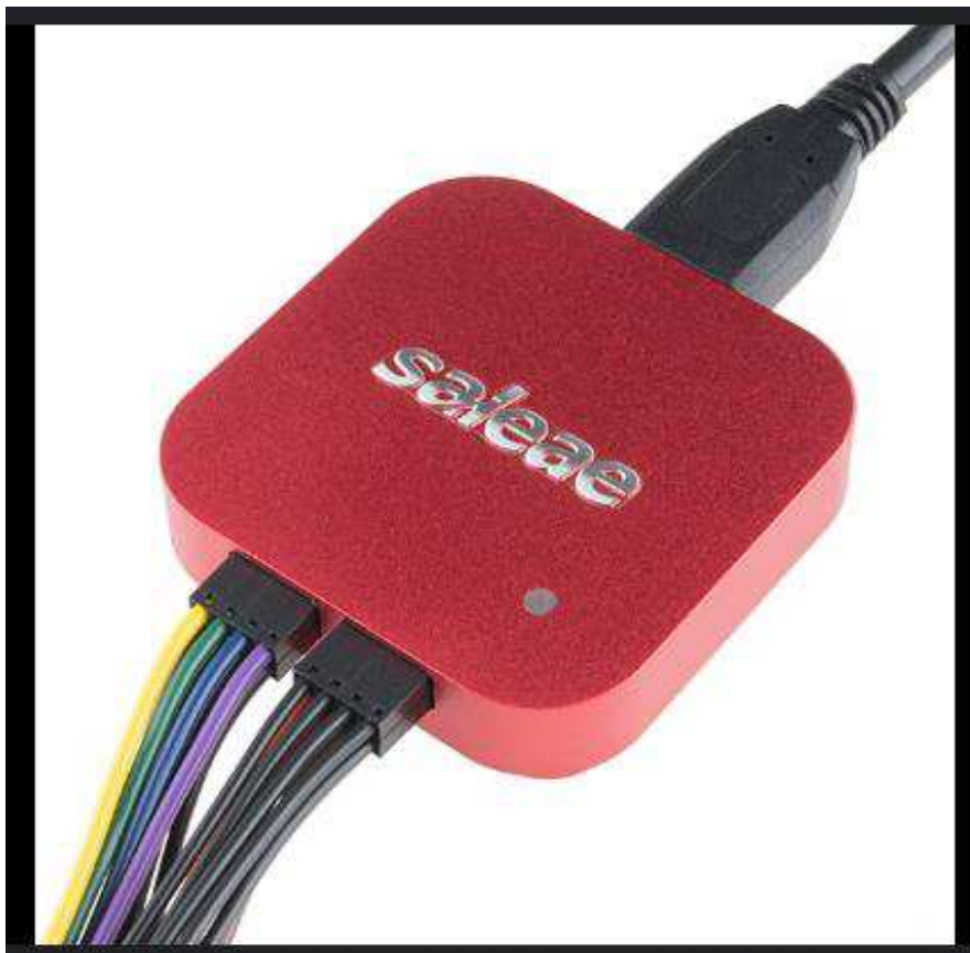
Slika 3: Saleae logic analyzer
