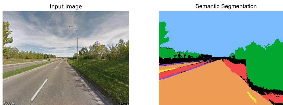
Figure 1.1: Example of road image being segmented into classes, where every color is a different class
