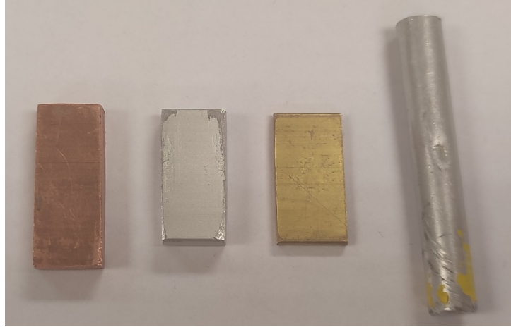
(b) Cuboids and PMA-1 landmine fuse (hollow aluminium cylinder).
