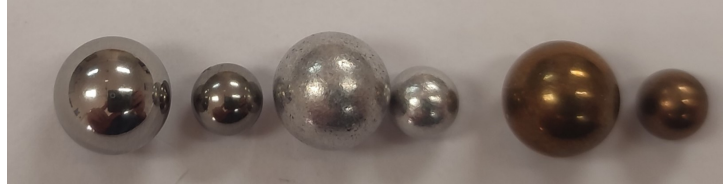
(a) Balls of different sizes (with diameters of 5 mm and 8 mm) and materials (stainless steel, aluminium, and brass).
