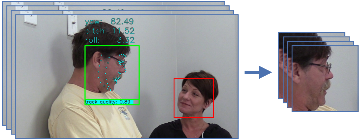
Figure 6.1: CCMiniVID video processing framework. All faces are tracked with a commercial tracking system. The metadata of multi-subject videos is manually filtered to contain only data related to the subject of interest. The framework extracts aligned face crop sequences using the raw CC videos and the produced tracking data.
