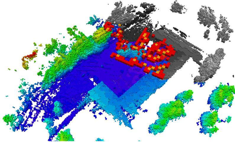
**Figure 4.6:** Results of mean-shift clustering during real-world experiments within this thesis. Grey and white parts of the OctoMap represent the unexplored and green/blue explored environment. Red voxels represent the frontier and yellow voxels are centroids of frontier point clusters, the output of the mean-shift algorithm.
