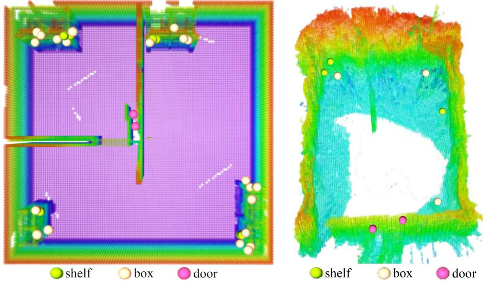
**Figure 4.14:** The OctoMap of the warehouse environment in the simulation and in the real-world experiment is shown on the left and right respectively. The transparency effect is applied on the OctoMap and detected objects during the exploration are shown. Shelves, boxes and doors are shown with different colors on the map.
