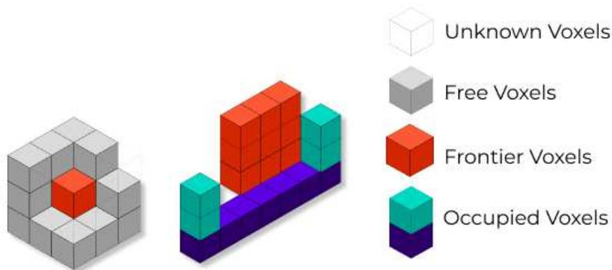
**Figure 4.3:** Illustration of a 3D frontier detection. The voxels are shown in 3D space which is a more complex, volumetric space where the boundary between free (gray) and unknown (transparent) voxels represents frontier (red) voxels.
