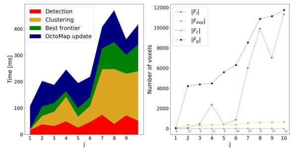
Fig. 6. House scenario metrics for  $r_{max} = 0.25$  m,  $r_{exp} = 1$  m, bandwidth = 2. On the left, the computation times for significant modules in each iteration  $j$  are shown. On the right, a graph shows the number of voxels in each iteration.
