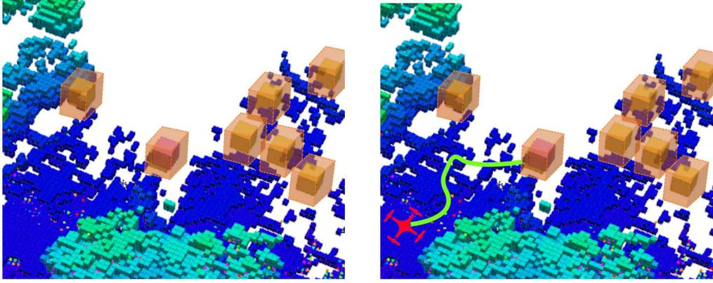
**Figure 4.7:** Information gain calculation for the potential exploration targets is shown on the left. Cubes are placed around the candidates and the information gain is proportional to the number of unknown voxels within the cubes. The UAV selects the best frontier according to Eq. 4.6, plans the path and navigates toward the target.
