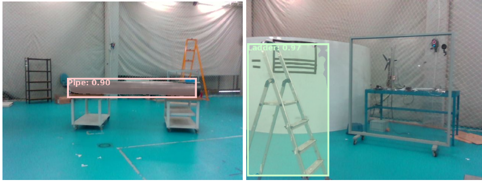
Figure 4.13: Results of the mmdetection algorithm using RetinaNet. The model, trained specifically for construction site environments, effectively detects pipes and ladders. The detection is performed in the real-world scenario.
