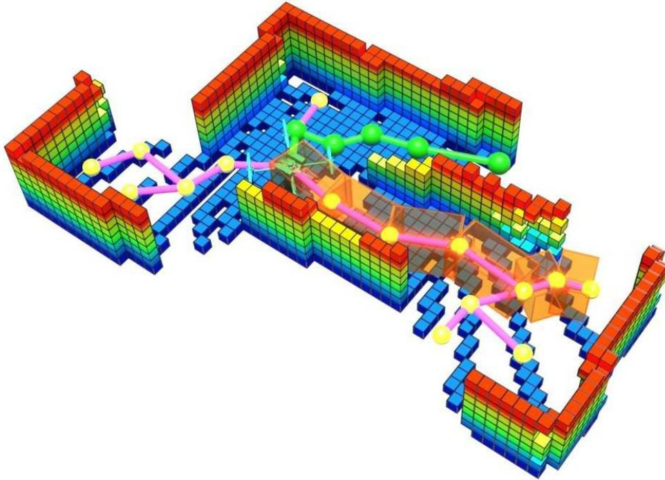
**Figure 4.11:** The UAV body (cyan color) denotes the first point of the path. Orange cuboids along the path of the RRT illustrate the volume where the information gain is computed. A green path with green waypoints is the best path. Pink paths with yellow waypoints are other paths of the RRT.
