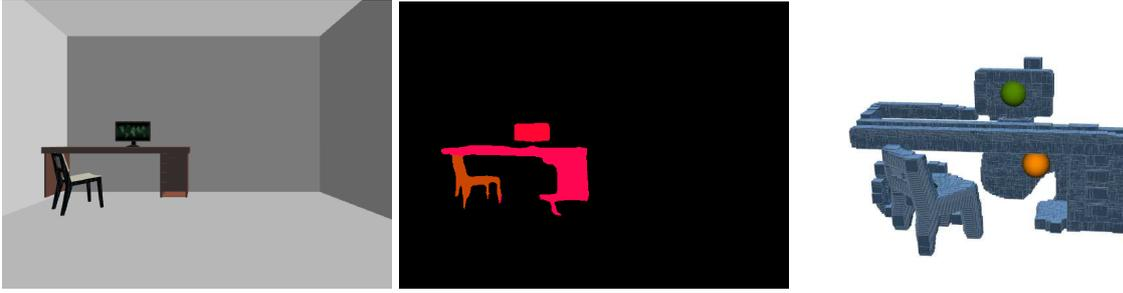
**Figure 4.12:** Semantic segmentation of simple features (table, chair and monitor). The semantic segmentation is performed with an HRNet model trained on the ADE20K dataset. Once the objects are semantically segmented, the 3D position of each object is extracted and colored in a specific color matched to the object.
