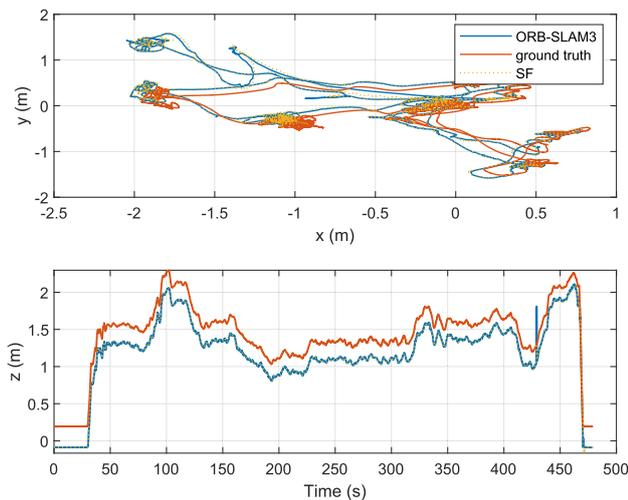
**FIGURE 17.** Comparison of ORB-SLAM3, multi-sensor fusion and ground truth positions for the  $x$ ,  $y$ , and  $z$  coordinates in a single exploration run.
