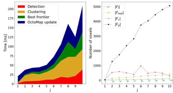
Fig. 8. Large scenario metrics for  $r_{max} = 0.5 \text{ m}$ ,  $r_{exp} = 2 \text{ m}$ , bandwidth = 2. On the left, the computation times for significant modules in each iteration  $j$  are shown. On the right, a graph shows the number of voxels in each iteration.
