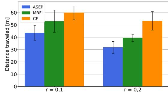
**FIGURE 11.** Total distance traveled in the simple environment for the ASEP, MRF and CF. Data are given as means of 10 runs with standard deviations.
