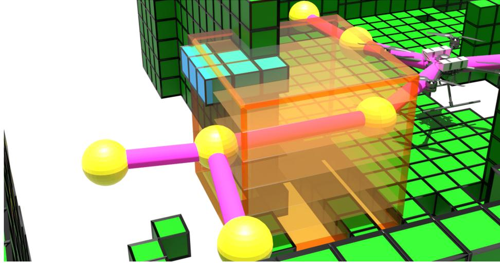
**Figure 4.10:** An illustration of the proposed Recursive Shadowcasting algorithm in the OctoMap. The algorithm is performed inside the cuboid centered at the path edge, on each 2D slice (planes inside the cuboid). The results of the RSC are shown on the first OctoMap slice, where the cyan voxels represent unknown voxels while the grey voxel is not taken into account for the information gain calculation.
