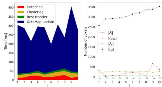
Fig. 13. Outdoor scenario metrics for  $r_{max} = 0.5\text{ m}$ ,  $r_{exp} = 2$ , bandwidth = 2. On the left, the computation times for significant modules in each iteration  $j$  are shown. On the right, a graph shows the number of voxels in each iteration.
