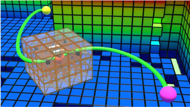
**FIGURE 3.** A UAV executes a planned path (green) from a start point (pink) to a target point (yellow) in an OctoMap. A rectangular prism-shaped state validity checker (transparent white and orange) simplifies the representation of the UAV. The validity checking is performed for each point (orange point) of the planned path.
