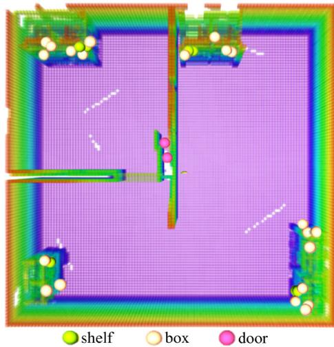
**FIGURE 7.** The OctoMap of the simple warehouse environment with transparency effect applied on and with detected objects during the exploration. Shelves, boxes and doors are shown with different colors on the map.
