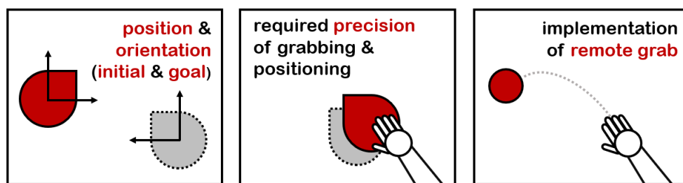
Figure 6.6: Examples of task-related parameters relevant for the implementation of pick-and-place mechanics (taken from [10])
