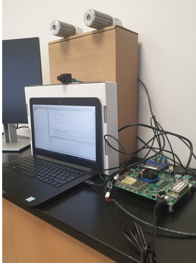
Figure 5.4: The image acquisition system setup including Xilinx ZCU104 board, OmniVision OV2311 image sensor, and two infrared illumination sources
