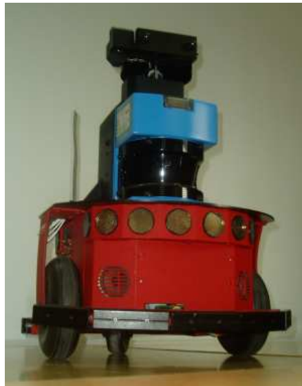
Figure 7.11. Pioneer 3DX mobile robot.
