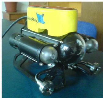
**Figure 3.7.** *VideoRay ROV with vision-based laser distance module.*
