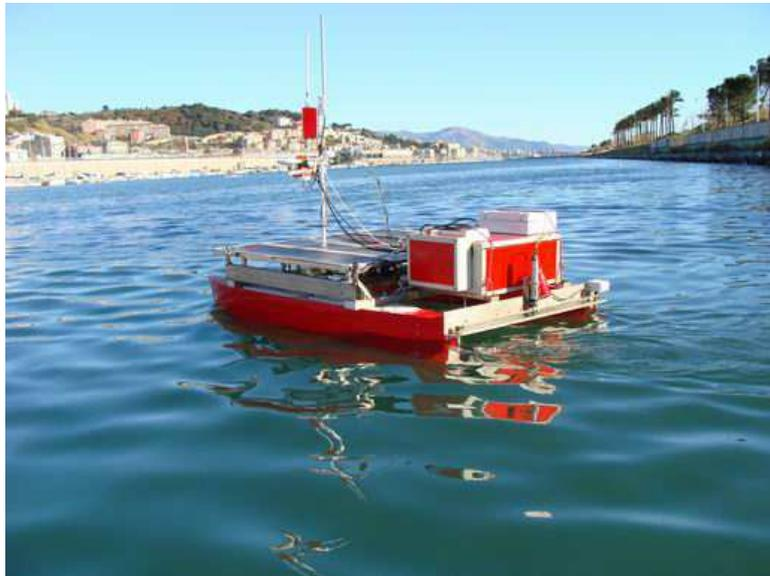
**Figure 3.6.** *Unmanned surface vehicle Charlie.*
