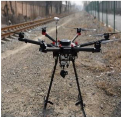
(c) Railroad inspection multirotor. Copyright [9] CC BY 4.0.
