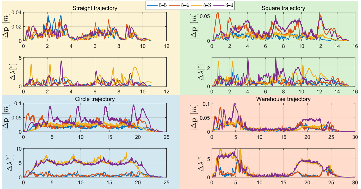
Figure 6.13: Position and orientation errors of the four benchmark trajectories, corrected and executed by four aerial manipulator combinations. Each benchmark trajectory is planned in the payload configuration, making it possible to achieve the same payload waypoints across different configurations. This allows for directly observing and comparing the errors. The perfect trajectory tracking is achieved when both position and orientation errors are zero.
