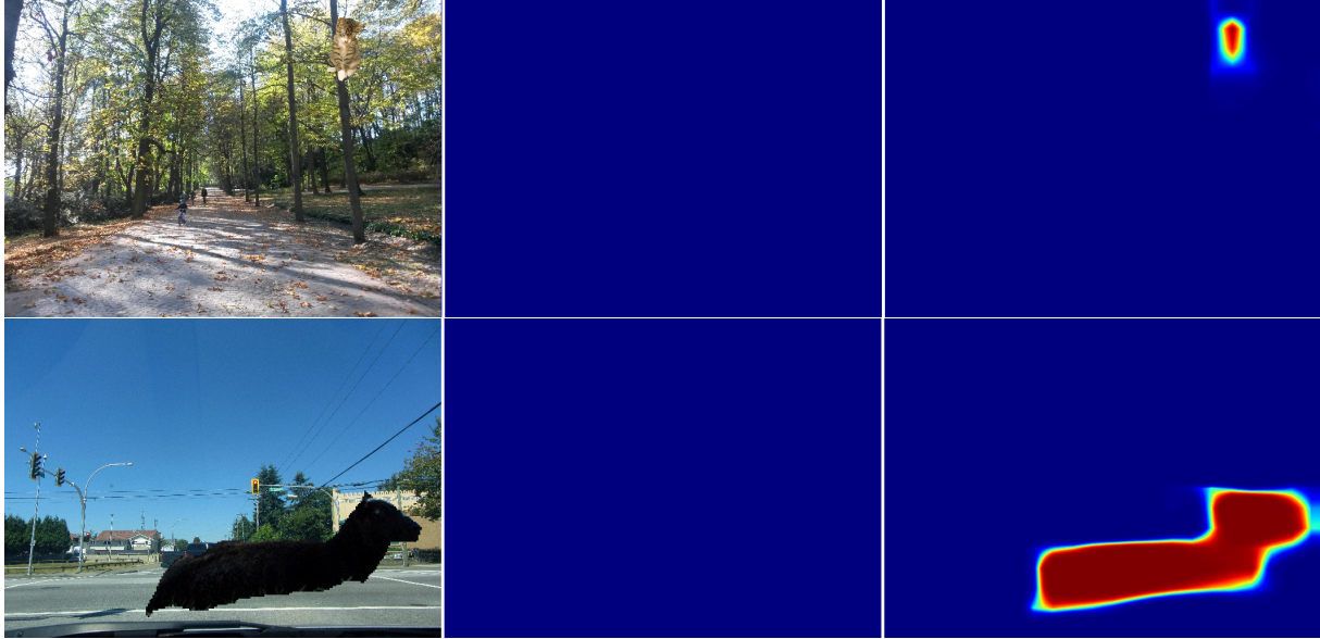
Figure 5.3: OOD detection in Vistas images with pasted Pascal animals. Row 1 shows a validation image from PascalVistas1, while row 2 presents an image from PascalVistas10. The columns correspond to: i) original image, ii) discriminative OOD detection trained without pasting and ii) discriminative OOD detection trained with pasting
