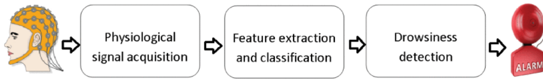
Figure 2.2 Block diagram representation of a typical physiological signal-based drivers' drowsiness detection system using EEG sensors. Source: [21] © 2018 IEEE
