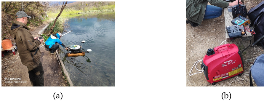
Figure 7.11: (a) Start of survey operations at lake Okrugljak. Two-person manual deployment of the ASV PlaDyBath from the shore of the lake. (b) Mission planning for the ASV PlaDyBath from a makeshift workstation.
