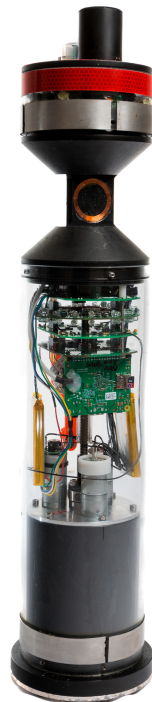
Figure 2.6: The aMussel underwater robot and sensor node. Note the inductive charging coils on the narrow neck below the top cap segment.
