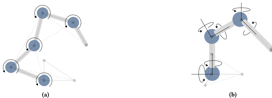
Figure 5.5: Visualization of planar and spherical mechanisms. These are two common examples of models for which our IK formulation uses a reduced number of variables.
