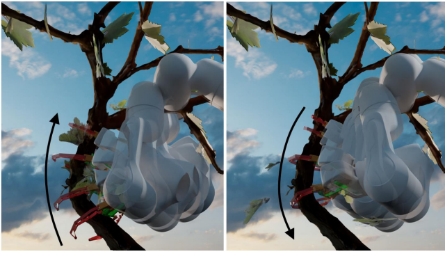
Fig. 2. Cleaning vine stems from scrubs and old rind starts with localizing and perching the plant proceeding to plant exploration moving upwards. Once we reach a certain threshold, the exploration stops, the grip is tightened and the cleaning procedure starts from the top.
