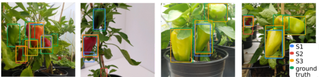
Figure 3.8: Pepper detection results on the real images from the test set. Ground truth human annotator labels are drawn in green. Results from networks trained on datasets S1 , S2 , and S3 , are shown in blue, red and yellow, respectively. Different learning results can be observed on different datasets.
