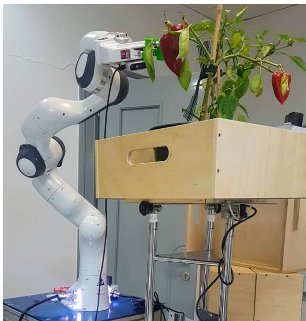
Fig. 1 Collaborative robot Franka Panda performing harvesting procedure on a sweet pepper ( Capsicum annuum ) plant in a controlled indoor farming setup
