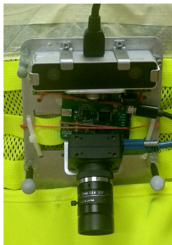
Figure 2.12: The visual sensor suite, stereo and monocular camera, upgraded with the UWB sensor.
