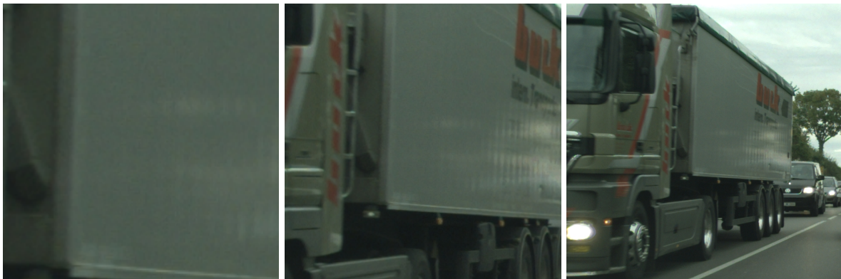
Figure 1.3: Pixels observed by a limited receptive field model across the resolution pyramid when inferring the class of the central pixel. Images (from left to right) are 1x, 2x and 4x subsampled.
