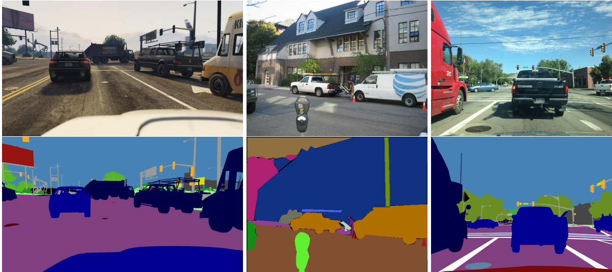
Figure 6.1: Example of inharmonious taxonomies for multi-domain semantic segmentation. Pickups are labeled as class truck in VIPER [120] (left), class van in Ade20k [101] (middle) and class car in Vistas [24] (right). We resolve the class overlap by learning on partial labels [119].
