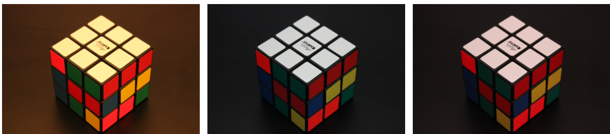
Figure 1.1: The impact of different white balance settings on the appearance of digital images. Images of the same scene are captured with three white balance settings. The settings used are the following: left image - Shade ; middle image - Tungsten light ; right image - White fluorescent light . All images were captured with the same Canon EOS 550D camera using ISO 3200, exposure time 1/15, and aperture f/5.6.
