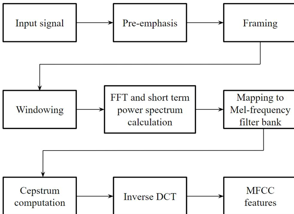
*Figure 4.4. Calculation flowchart for Mel Frequency Cepstral Coefficients*
