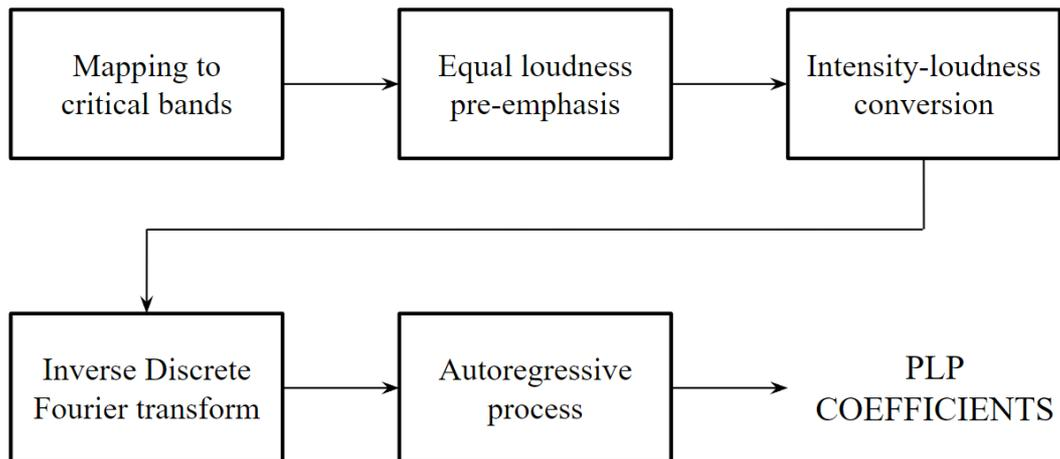
*Figure 4.5. Calculation flowchart for Perceptual Linear Prediction coefficients*
