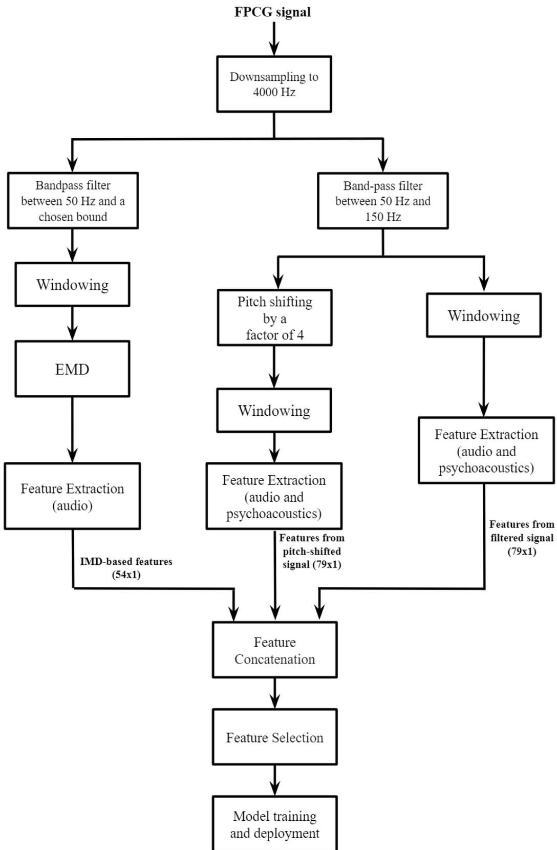
*Figure 5.1. Block diagram of the overall proposed algorithm for FPCG signal classification.*
