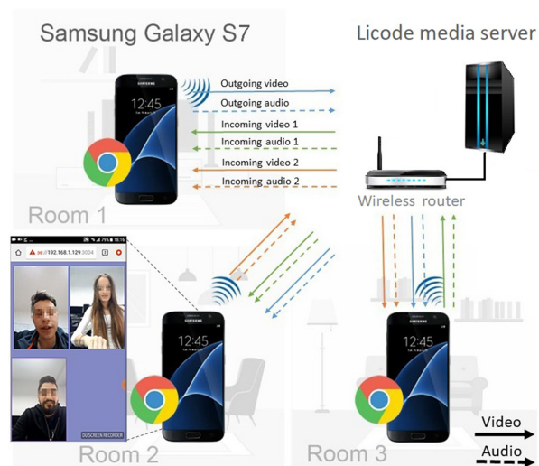
Figure 5.10: Testbed set-up over a LAN connection (user study US5).
