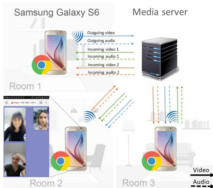
Figure 6.8: Testbed set-up over a LAN (user study US4).
