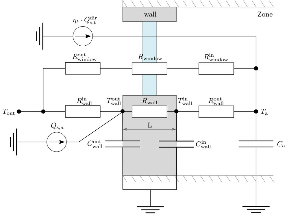
**Figure 3.3.** An analogous RC network model of an external wall with a window.
