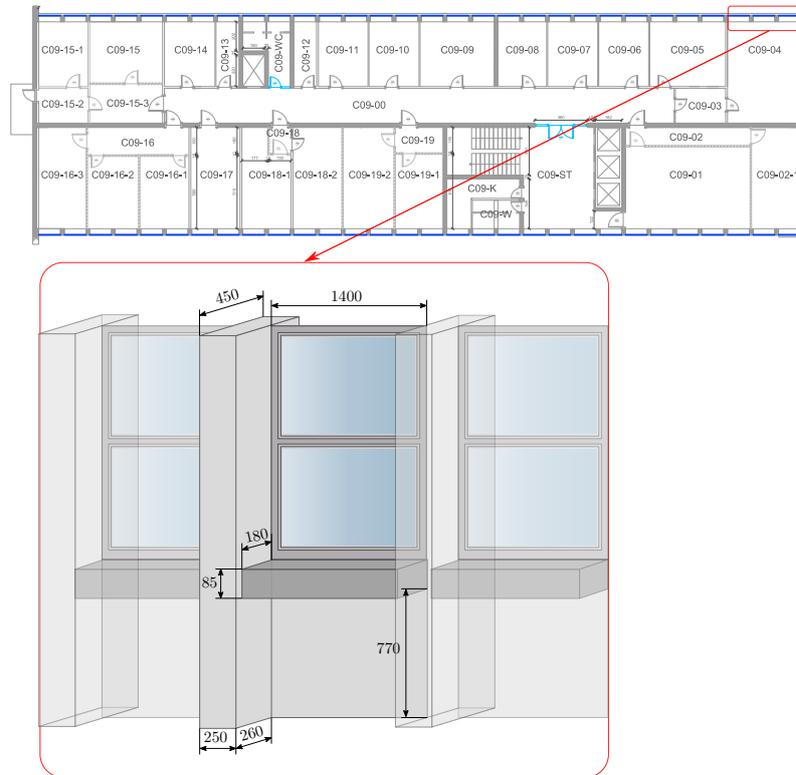
**Figure A.7.** Reinforced concrete columns on south- and north-facing sides of the building.
