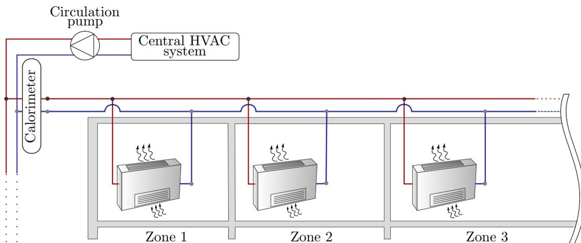
**Figure 2.1.** *Illustration of a system of FCUs.*
