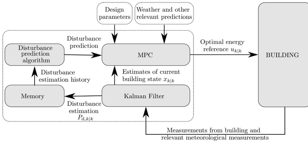
**Figure 5.4.** MPC control scheme for offset-free zone temperature control.
