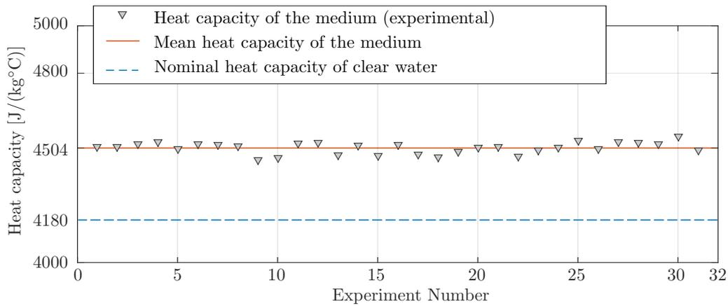
**Figure 2.13.** Identified heat capacity of the heating/cooling medium.
