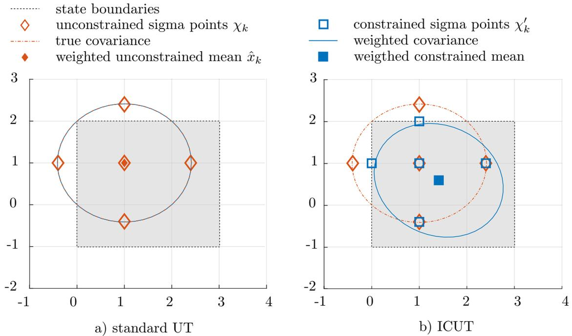
**Figure 3.7.** Geometrical interpretation of the proposed modified ICUT.
