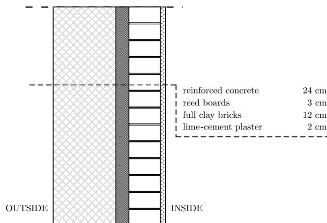
**Figure A.6.** East- and west-facing external walls from the ground floor to 13<sup>th</sup> floor (EW2).
