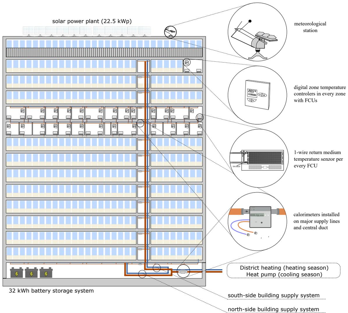
**Figure A.2.** *Equipment installed in UNIZGFER building.*
