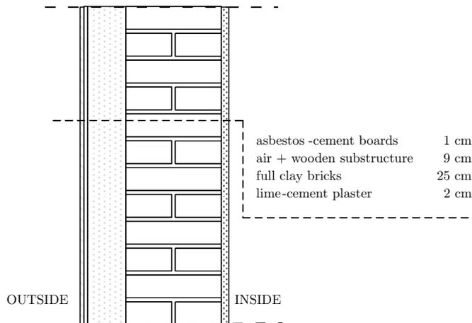
**Figure A.8.** South- and north-facing external walls from ground-floor to 12<sup>th</sup> floor (EW3).
