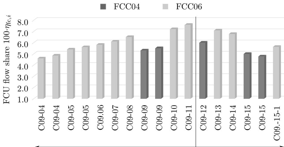
**Figure 2.12.** Flow distribution of the medium mass flow among FCUs connected to south supply line on the 9<sup>th</sup> floor.
