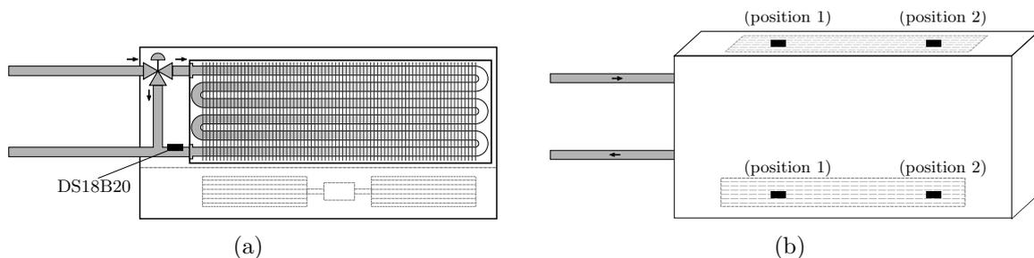
**Figure A.4.** a) FCU installation with three-way valve and 1-wire return medium temperature sensor DS18B20 mounted on the return pipe, b) placement of additional 1-wire DS18B20 sensors for monitoring incoming and outgoing air temperatures.
