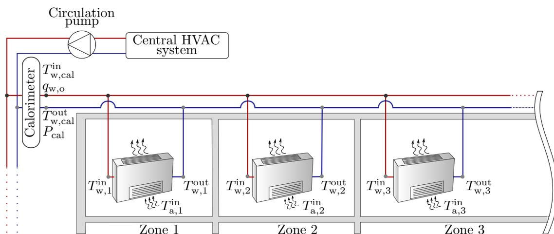
**Figure 2.4.** Considered configuration of a system of FCUs.
