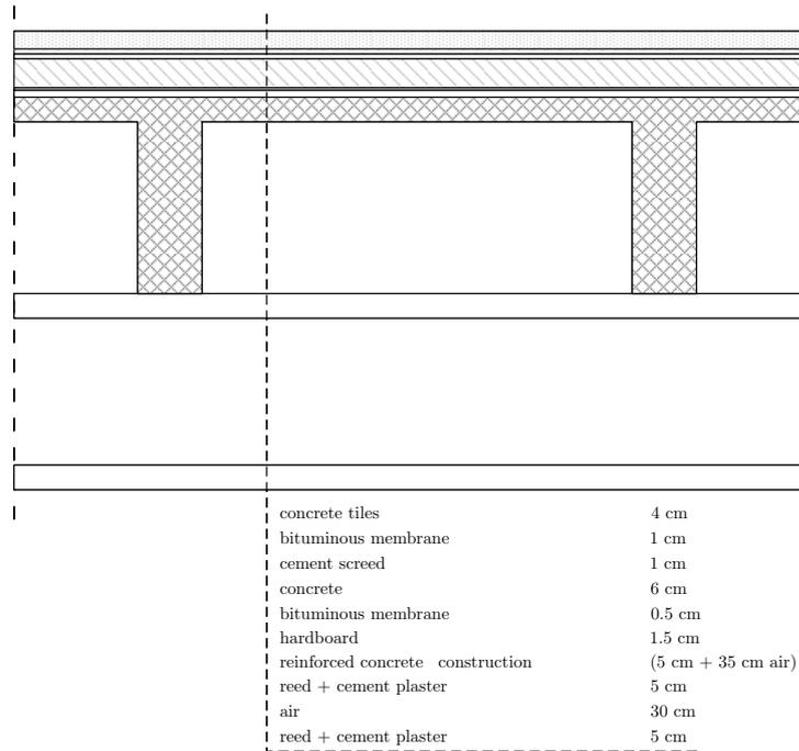
**Figure A.19.** Ceiling on the 12<sup>th</sup> floor (FC5).
