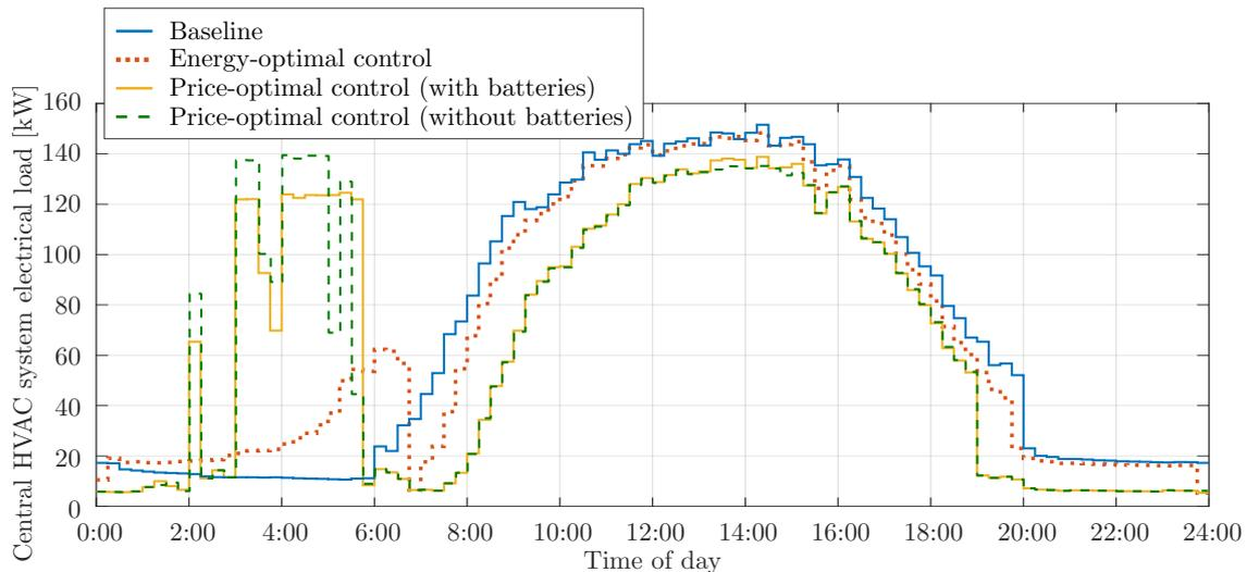
**Figure 6.15.** Central HVAC system electrical load profile average in 15-minute time instants obtained with different control strategies.
