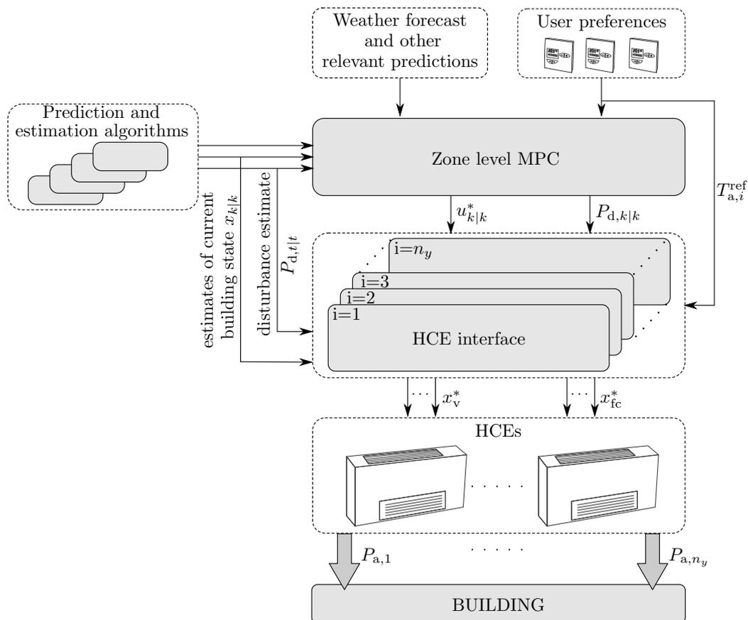
**Figure 5.18.** Hierarchical MPC for zones comfort control.
