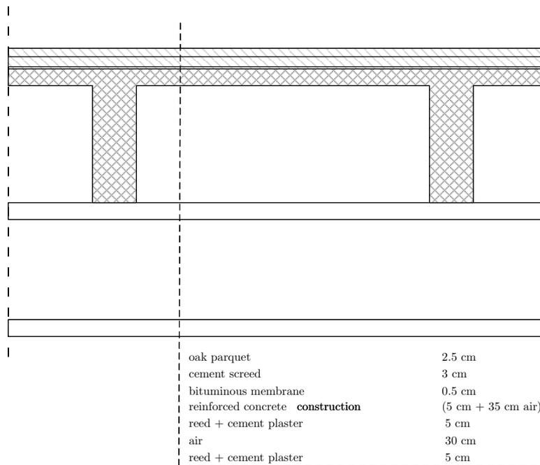
**Figure A.18.** *Ceiling on the 12<sup>th</sup> floor (FC4).*
