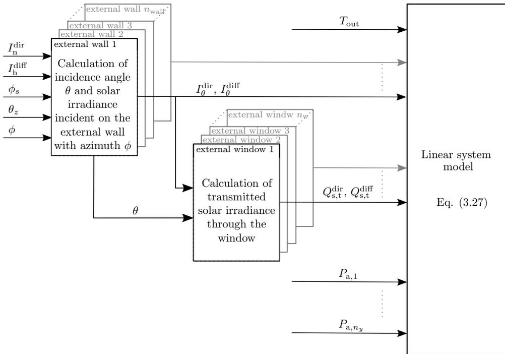
**Figure 3.6.** Preprocessing of nonlinear solar irradiance effects.
