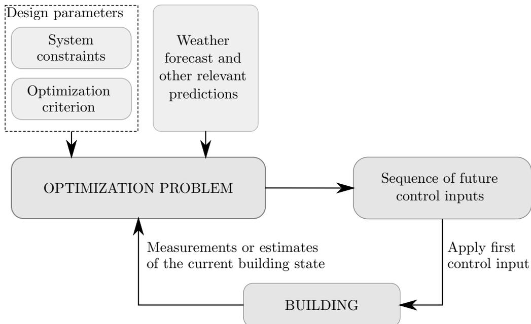
**Figure 5.1.** MPC scheme for building comfort control.
