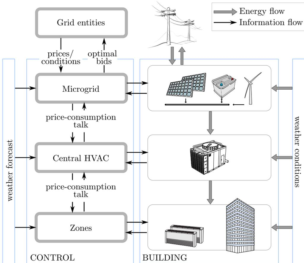
**Figure 6.1.** Modular control of main building subsystems.
