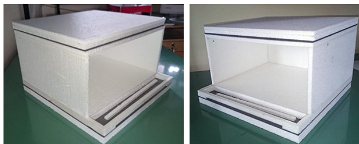
FIGURE 2.20. Photography of scaled mock-up with EPS and bitumen elements
