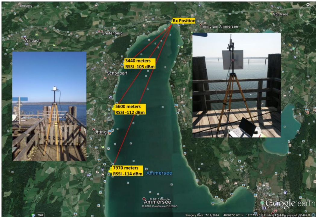
Figure 5.6. Range tests at lake Ammersee (south Germany) with the ~ 8 km achieved transmission range. The data logger module was equipped with the high gain antenna shown on the right (+12.5 dBi) and the sensor module (shown on left) with the integrated PCB antenna (~ 0 dBi).
