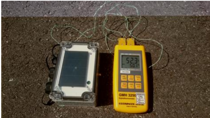
Figure 2.23. Measuring temperature inside a sensor module housing. The two channels of the thermometer (yellow device) are measuring the temperature of the solar cell (52.3 °C) and supercapacitor (50.1 °C) respectively. Outside temperature was 30 °C.
