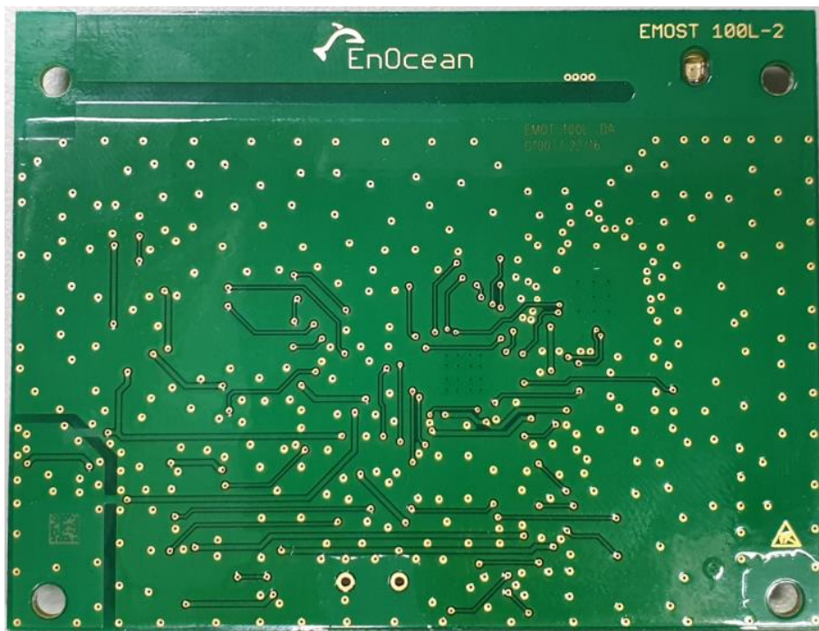
Figure 2.64. Assembled data logger module PCB (bottom view).
