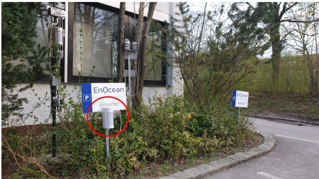
Figure 5.14. “Always ON” infrared sensor for parking occupancy monitoring. Sensor is attached to the left of the parking sign and connected to a sensor module placed on a pole in the background with the solar cell facing towards building. Another infrared sensor can also be seen on the pole above, together with some other sensors. This is the second test site in south Germany.
