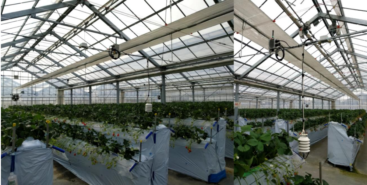
Figure 5.21. A sensor module installed in a greenhouse to monitor conditions during strawberry growth.
