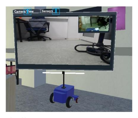
**Figure 3.2:** Front and back camera view on the panel above the robot.
