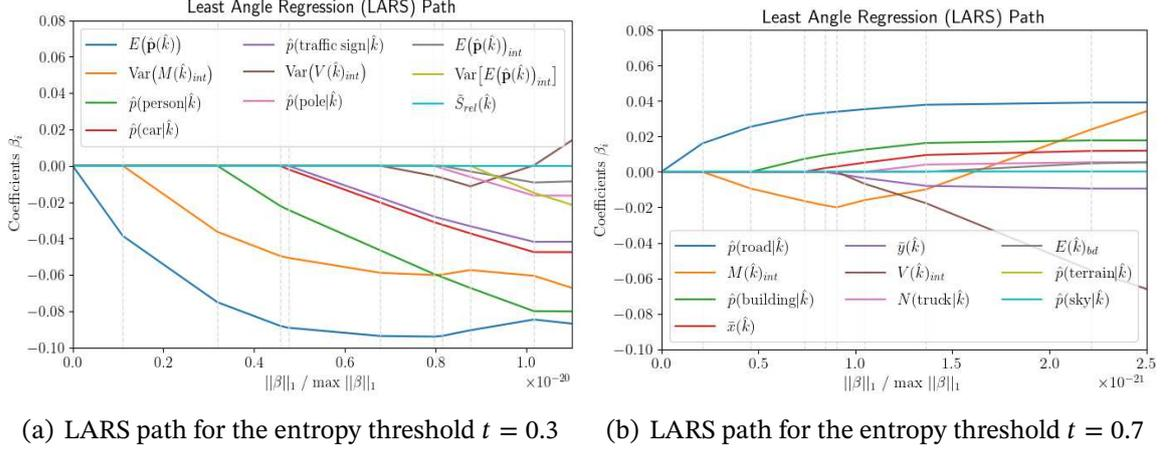
**Figure 5.6:** LARS paths for the hand-crafted metrics constructed from the output of a semantic segmentation network. Note that we apply LARS on the hand-crafted metrics obtained with the entropy threshold  $t = 0.3$  and  $t = 0.7$  and display the top ten hand-crafted metrics most correlated with the response of logistic regression. A detailed description of the hand-crafted metrics can be found in [12].
