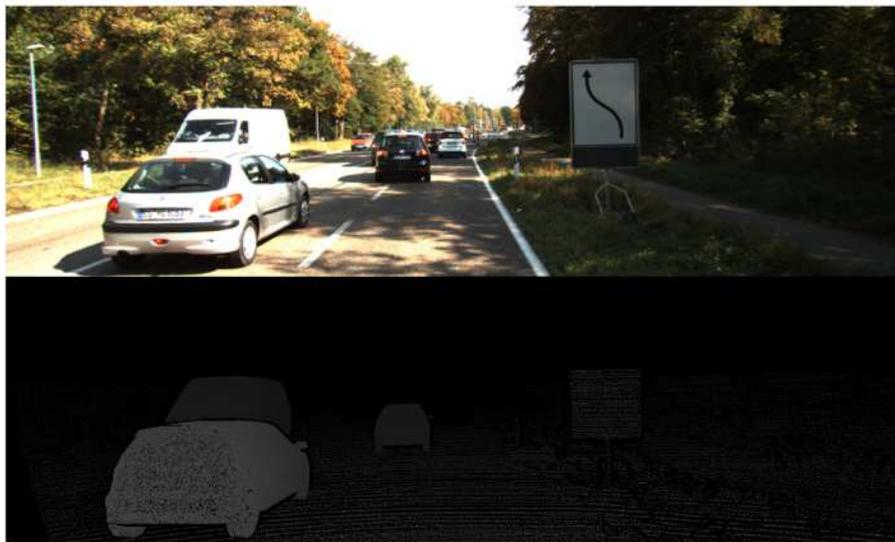
**Figure 6.1:** An example from the KITTI 2015 dataset. The top image shows the reference left image, and the bottom image shows the corresponding disparity map obtained by a laser sensor.
