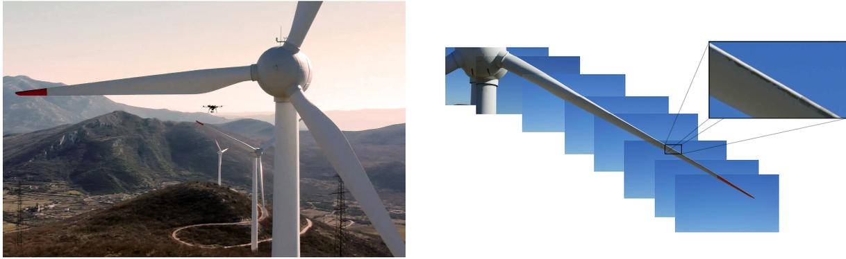
**Figure 2.2:** Autonomous wind turbine inspection conducted by an UAV (left). High-resolution images acquired during the survey mission that are used for damage assessment on the wind turbine blades (right).
