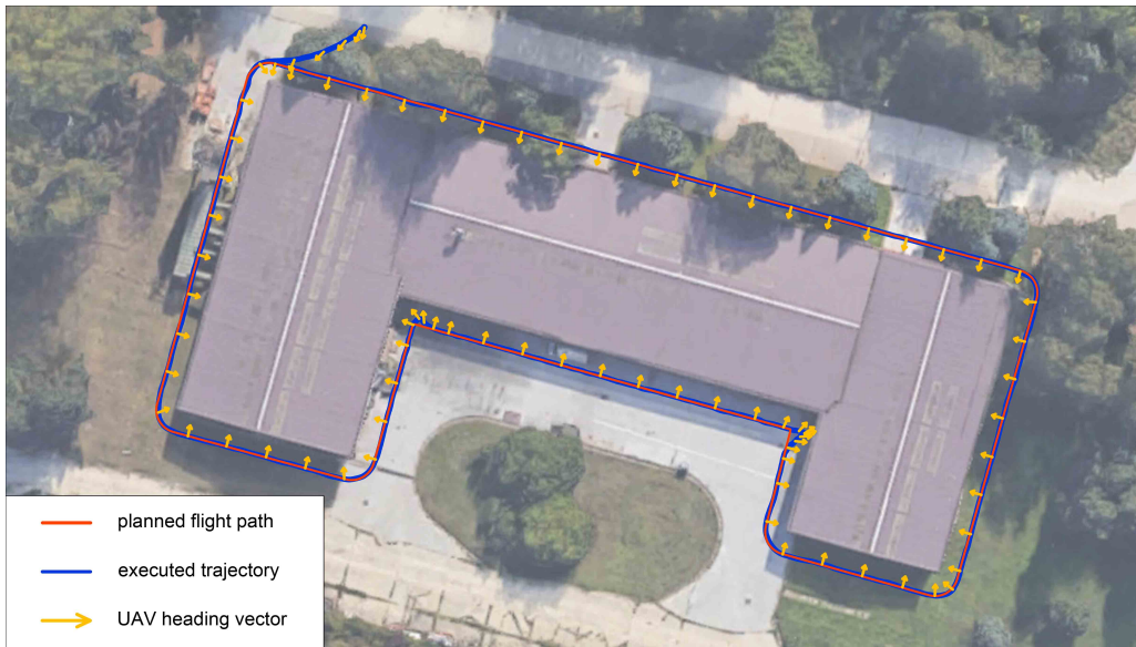
Figure 4.9: Planned flight path, executed trajectory and UAV's heading vectors in experimental surveying of the test site building.
