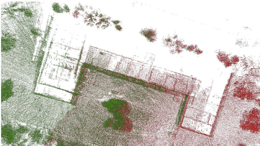
**Figure 4.10:** This image shows a top-down view of the map obtained using the acquired data from two different UAVs performing a data-acquisition scenario. Green and red points represent the map obtained by UAV-1 and UAV-2 respectively.
