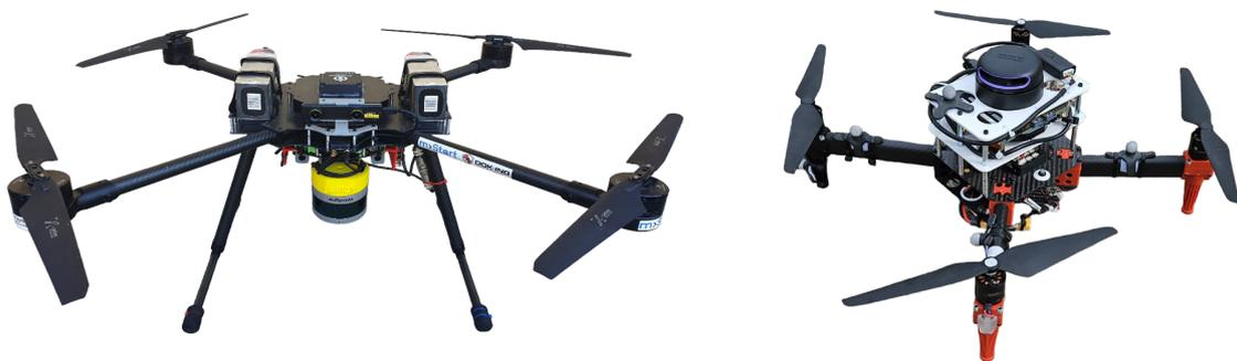
**Figure 3.7:** Quadcopters used in experiments - *Kopterworx* UAV with equipped *Velodyne VLP-16* LiDAR sensor and *ZED* stereo camera (left), and modified *Hexsoon EDU-450* with *SLAMTEC RPLIDAR-A3* 2D LiDAR used for obstacle detection (right).
