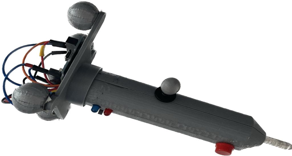
**Figure 4.4:** The functionalities of a wireless joystick and a virtual marker were combined to design a prototype of an active virtual pen that can be used to program and deploy robotic systems.
