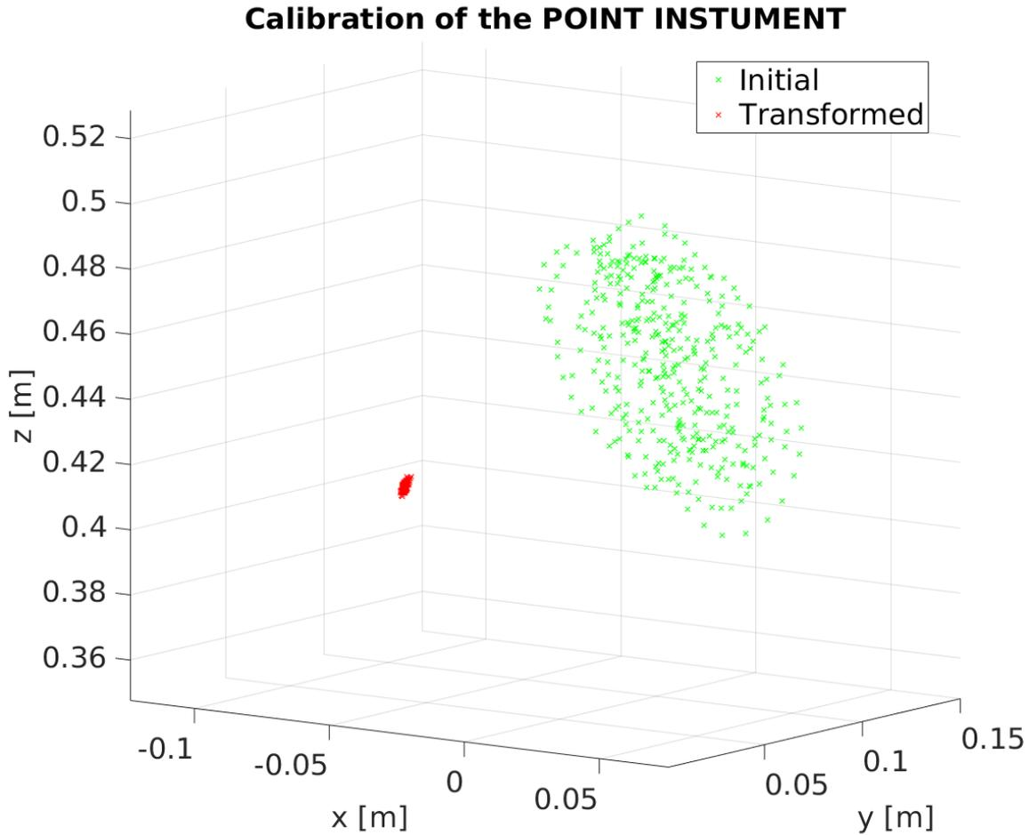
**Figure 4.8:** Figure shows result of  $T_I^P$  optimisation process. The recorded points of the centroid  $T_0^I$  are presented in green, while final transformation of the instrument tip  $T_0^P$  is presented in red.
