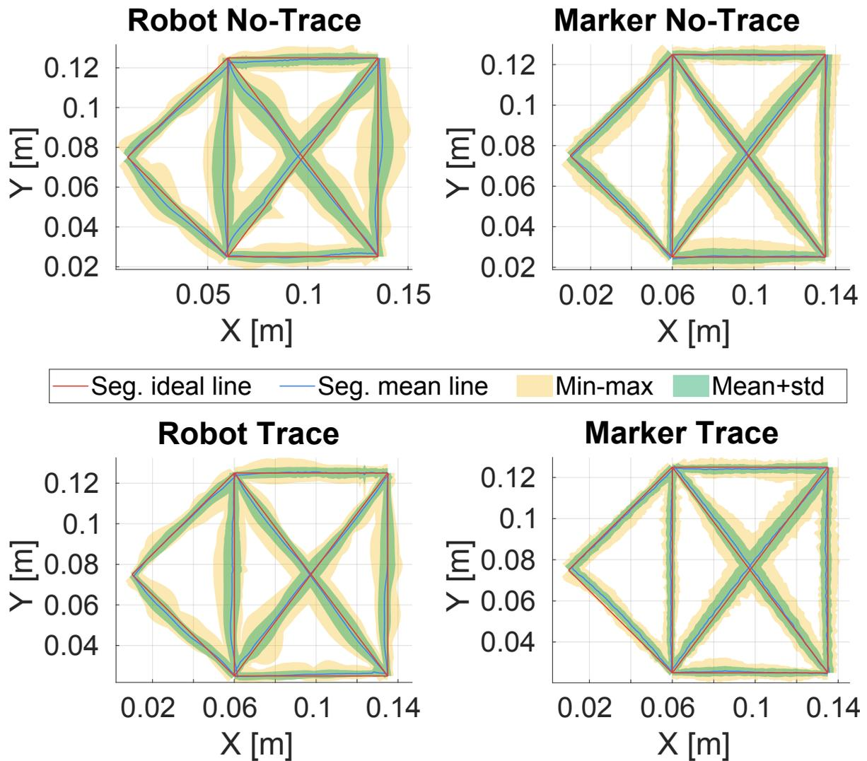
**Figure 4.16:** The illustration showcases demonstrated trajectories, with the ideal trajectory highlighted in red. The blue line depicts the mean value, derived from distances between the points of trajectories and their respective orthogonal projections onto the ideal segment line. Yellow indicates the range between minimum and maximum trajectory values, while the green area portrays the standard deviation from the mean trajectory.
