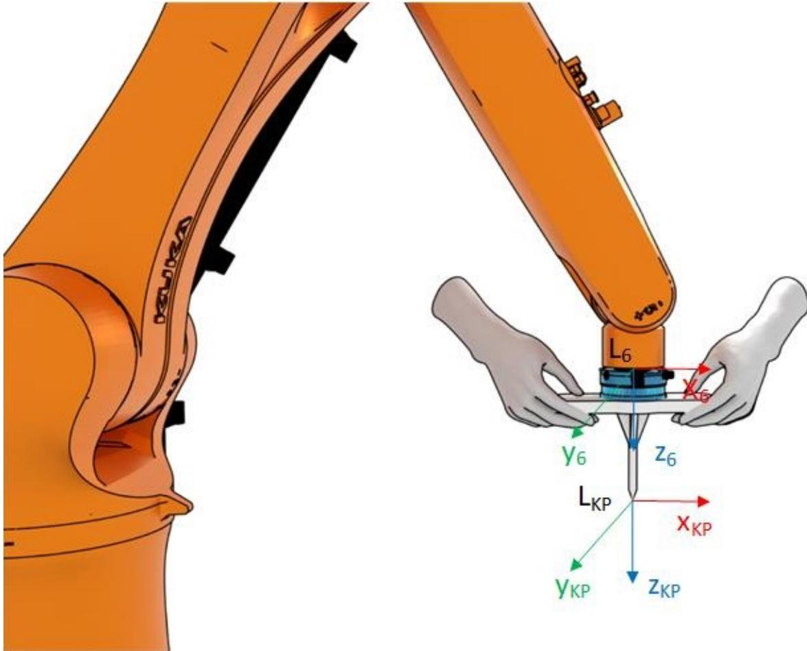
**Figure 4.10:** Showing KUKA KR10 robot equipped with point-tip for point measurement. The robot has collaborative behaviour due to the installed force sensor between the pin tool and robot flange, and collaborative force control system. The operator takes pin tool holder and moves robot towards point of the interest. After positioning measurement pin, robot pose is captured and used for global position measurement.
