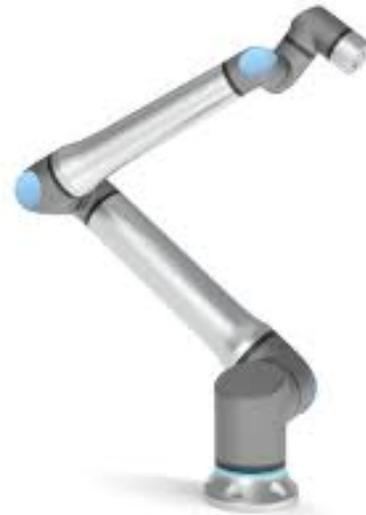
(b) Collaborative: Universal Robots UR20 <sup>2</sup>**Figure 1.1:** Robot manipulators
