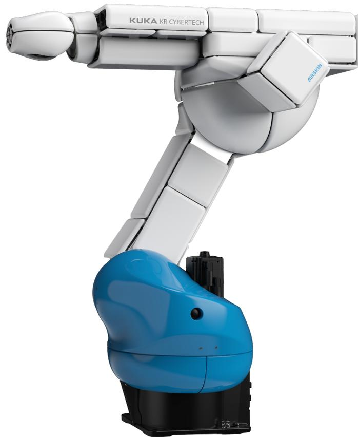
**Figure 5.4:** *AIRSKIN*<sup>®</sup> safety system, consisting of air pockets that are put on each link of the robot. When in contact, pressure disturbance within a single pocket triggers an emergency state.
