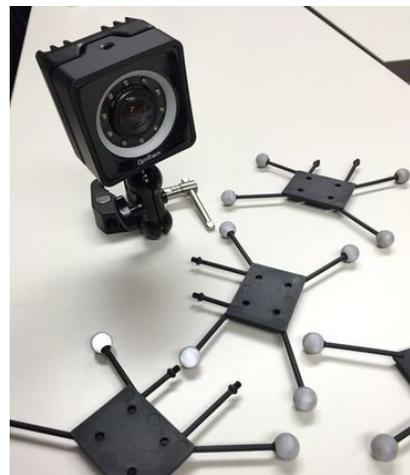
(c) Optitrack markers and camera <sup>7</sup>
