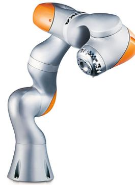
(b) KUKA iiwa <sup>4</sup>**Figure 4.2:** Collaborative robot manipulators
