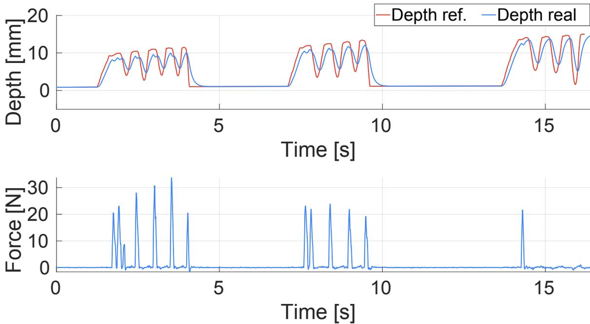
**Figure 6.15:** Drilling of a 15 mm hole with the robot using the DMP obtained from human motion recording. The drilling feed rates typically reach up to 300 mm/min, while the service feed rates typically reach up to 3.000 mm/min. The drilling forces reach up to 30N.
