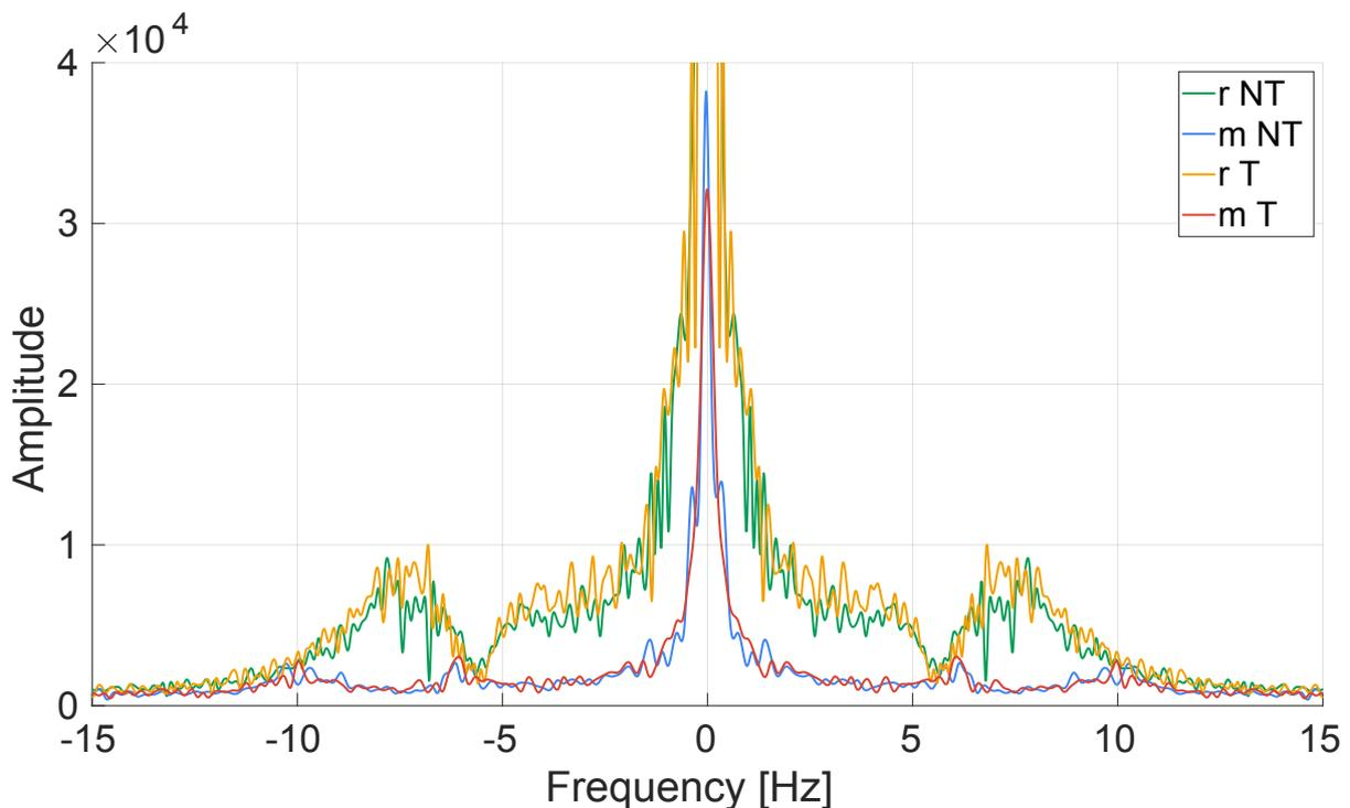
**Figure 4.18:** Fast-Fourier-Transformation of force signals. Demonstrations where marker does not leave trace are shown in green (robot) and blue (marker), while yellow (robot) and red (marker) denote demonstrations with the marker that does leave trace.
