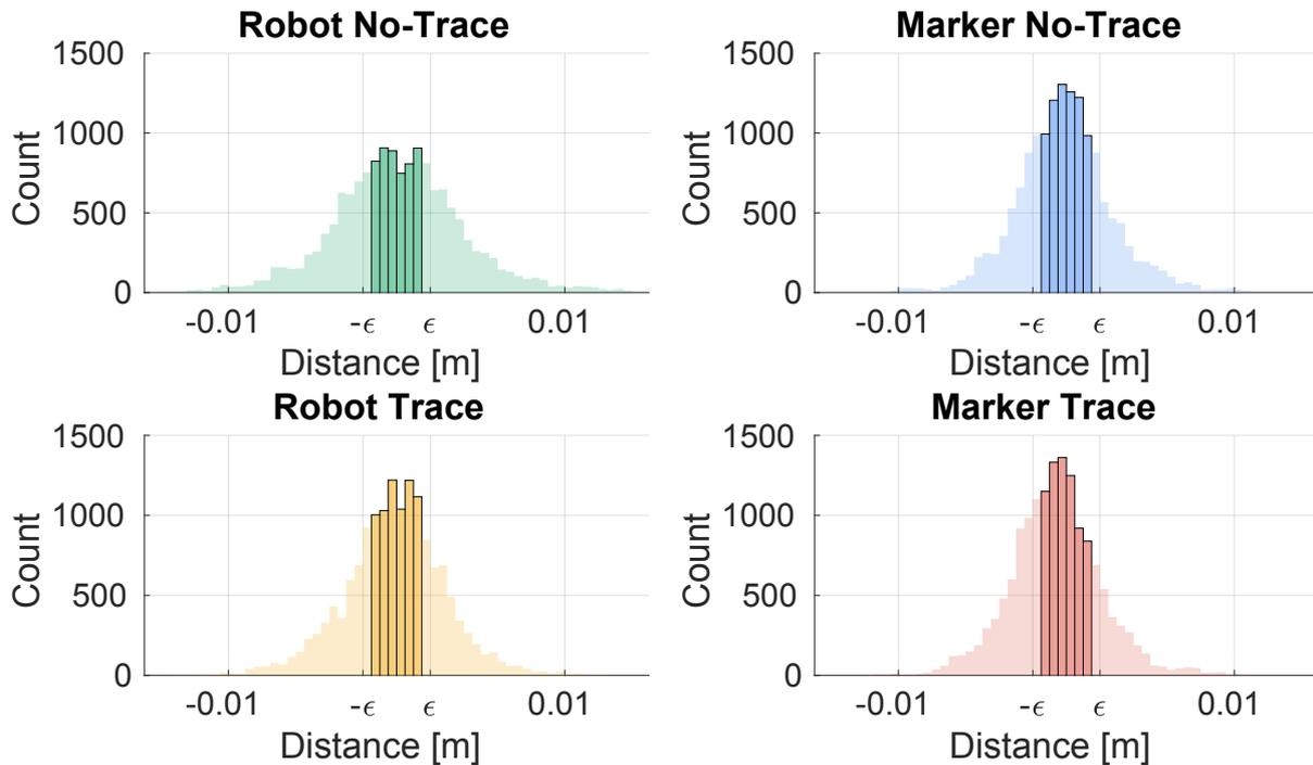
**Figure 4.17:** Distribution of distances of trajectory points from the ideal segment's lines, accompanied by the corresponding count of such points. The narrow  $\epsilon$  area, indicating where the majority of well-demonstrated trajectory points are expected, is highlighted.
