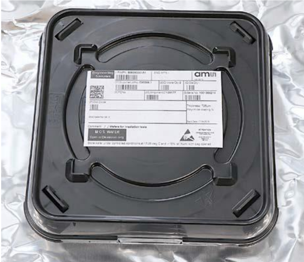
Figure 4.6. Wafer box containing the wafer for X-ray irradiation experiments. The contents of the box also include protective sponges and plastic layers in order to fixate and immobilize the wafer during its transport.
