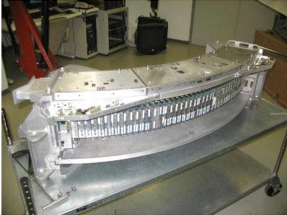
Figure 1.4. Philips 8-cm data measurement system, composed of multiple detector array modules [20].
