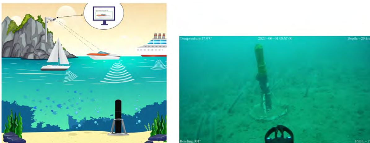
Figure 3. Setup of the recorder. Left panel: Illustration of the acoustic-optic testbed for quantifying the URN of VOO by using synchronized optical measurements from a shore based camera and an acoustic recorder positioned at the seabed. Right panel: Picture of the underwater acoustic recorder at the deployment site.
