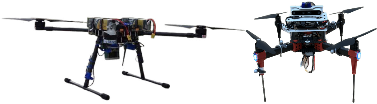
Figure 1.2: UAVs used in outdoor and indoor experiments. On the left is a Kopterworx quadcopter, a custom built quadcopter equipped with a Velodyne VLP – 16 LiDAR sensor. On the right is a Hexsoon EDU-450 quadcopter equipped with a Realsense D455 camera.
