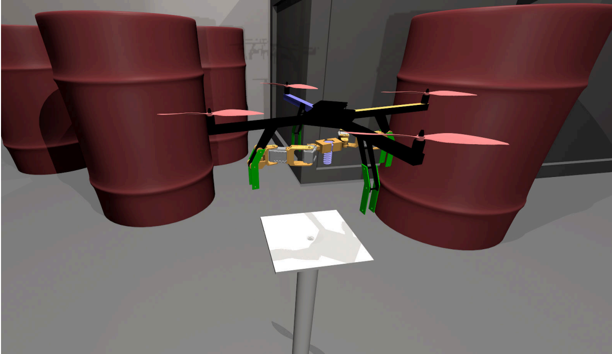
Figure 7.11: Image shows a mockup environment where a UAV equipped with a multi degree of freedom dual arm manipulator inserts a peg (screw) in hole (stand with the designated insertion hole). The proposed system can be applied to various scenarios including, but not limited to maintenance, inspection or repair missions.
