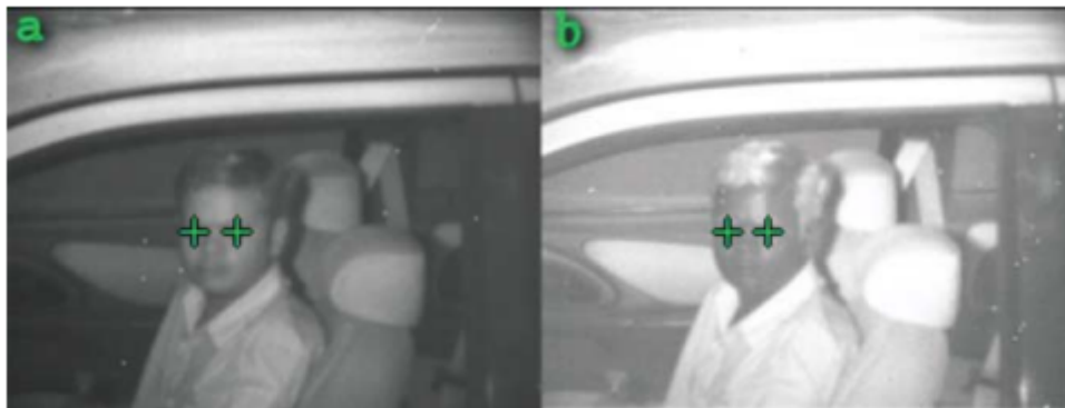
Figure 3.17: Algorithm execution for detecting eyes in lower NIR band image (a) and higher NIR band image (b) [95]
