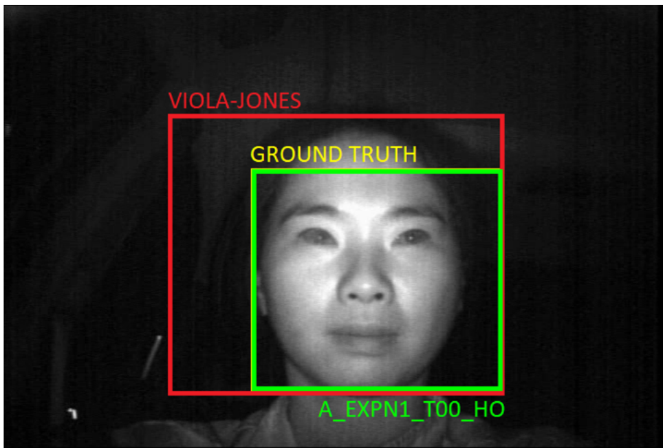
Figure 4.9: Successful detection example with ground truth face region bounding box (yellow), proposed variant A_Expn1_T00_HO face region bounding box (green), and Viola-Jones face region bounding box (red)
