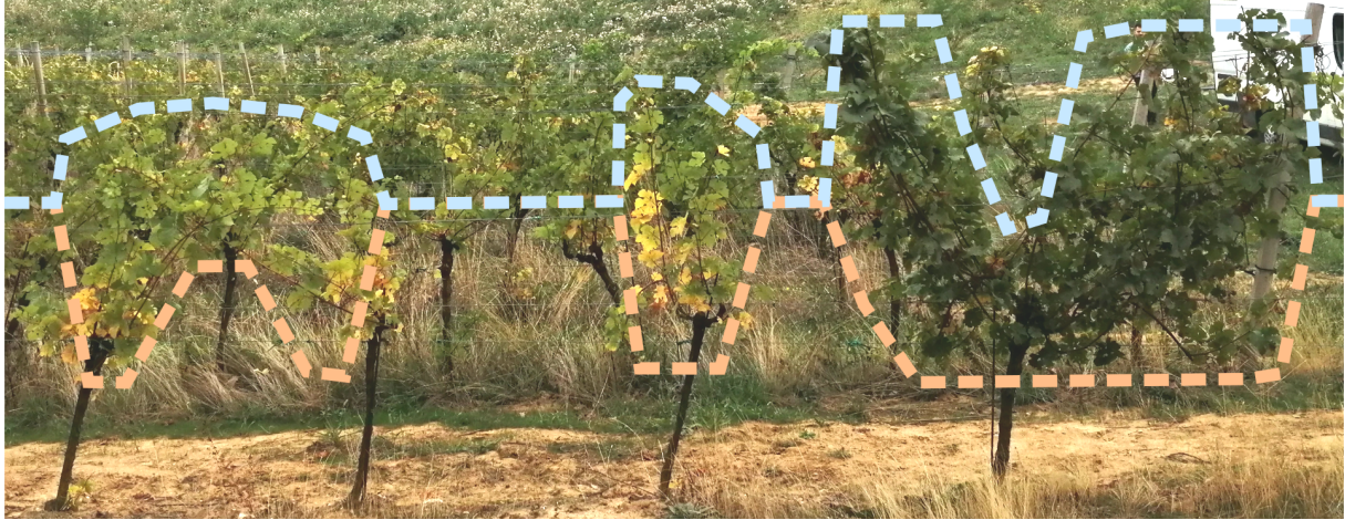
Figure 3.7: The canopy description used for the continuous spraying experiment in a vineyard, selected by an operator using a simple graphical user interface. Copyright [8]CC BY 4.0.
