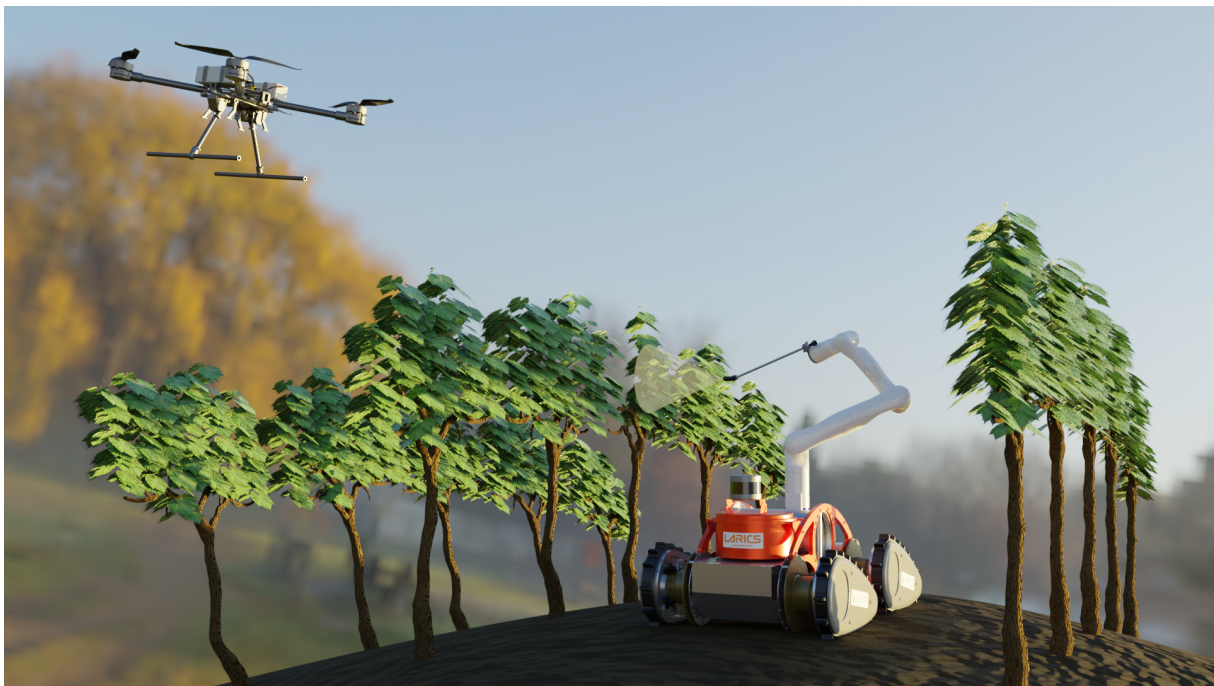
Figure 1.1: A visualization of the heterogeneous robotic system employed in a vineyard as a part of the HEKTOR project, consisting of an unmanned aerial vehicle and an autonomous mobile manipulator.
