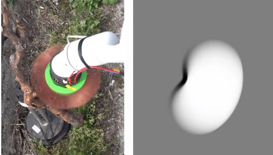
Figure 4.15: Occupancy grid mapping at a constant tool height during the suckering experiment. The map is built online, being constantly updated during the experiment.
