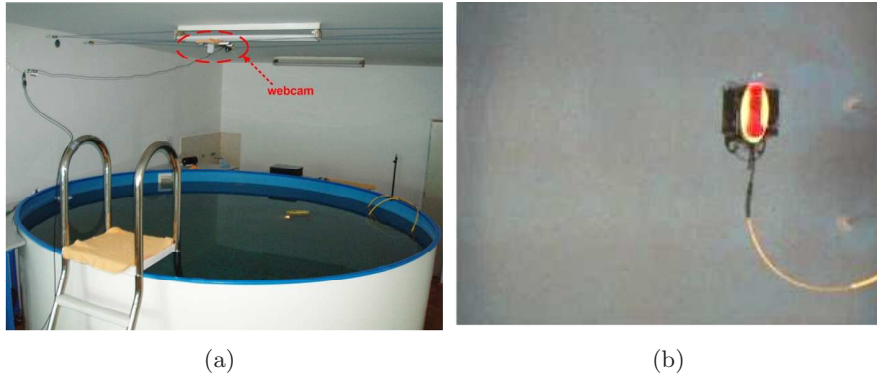
Figure 3.12. a) Laboratory setup for marine vehicle model identification and b) an acquired image from the camera placed above the pool.
