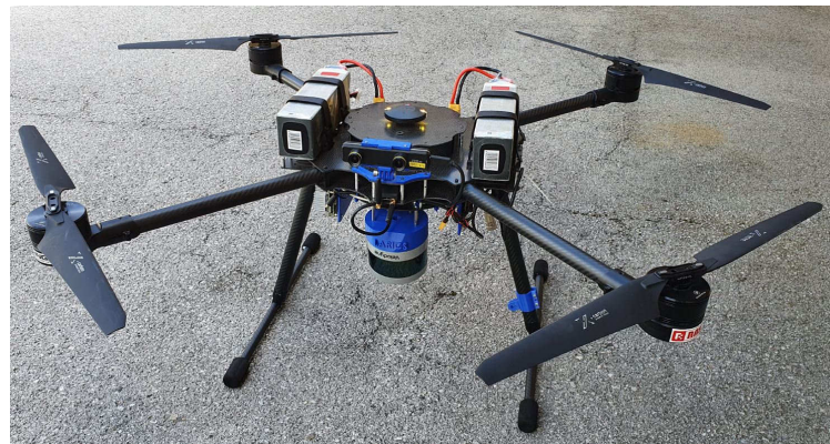
(d) Wind turbine inspection multirotor. Copyright [7] CC BY 4.0.
