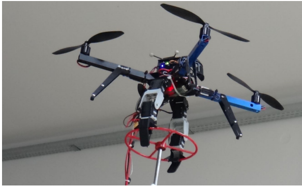
(a) Valve turning experiment. ©2014 IEEE. Reprinted with permission from [29].
